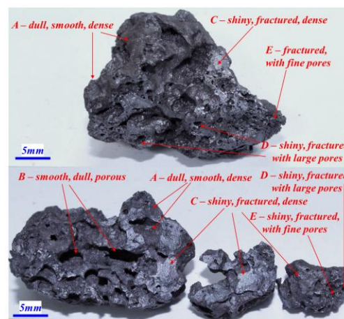
Figure 1 Macro-type features A-E on sinter particles [6]
