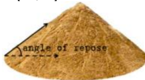
Figure 29: Angle of Repose Representation [101]
