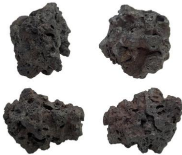
Figure 1: Images of an irregularly shaped sinter particle [20]
