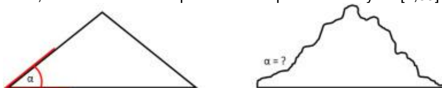
Figure 30: 'Ideal' vs. 'non-ideal' conical heaps of bulk material [101]
