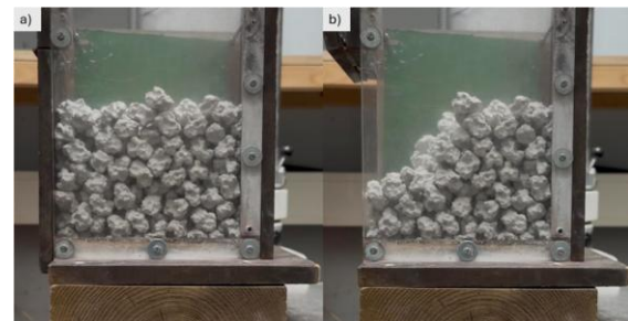
Figure 7: Ledge box: a) front gate closed; b) front gate open
