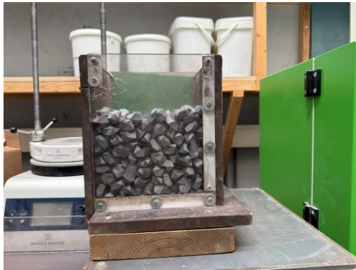
Figure 33: Filled ledge test box, with 40-face particles
