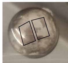
Figure 3.19. Image of the lens after ICP RIE. In the image, the arrays are outlined.
