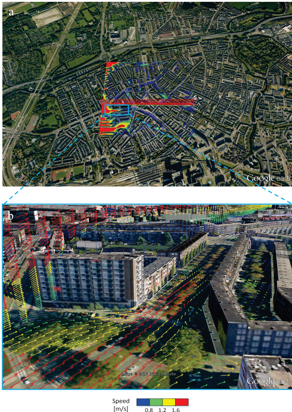
Figure 7. Vector representation of the wind flow in characteristic horizontal (close to the ground) and vertical planes: (a) overview for the entire domain at z = 1 m and y = 454 m planes; (b) zoom-in. The street-canyon effect (in the horizontal plane) and wakes generated behind taller buildings (in the vertical plane) can be easily observed. Note: a length of 12 m represents the reference vector of 2 m/s.
