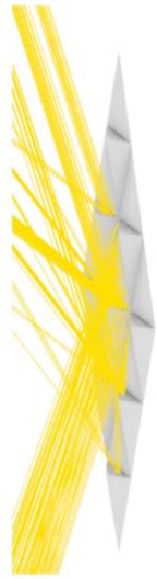
3) reflected rays: 60% on June 21 st 12hrs 85% on June 21 st 10–18hrs
