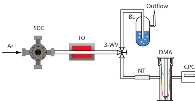
**Fig. 1.** Schematic layout of the experimental setup used for the synthesis and characterization of the test AgNPs. Key: SDG, spark discharge generator; TO, tube oven; 3WV, three-way valve; BL, bubbler; NT, aerosol neutralizer; DMA, differential mobility analyzer; CPC, condensation particle counter.
