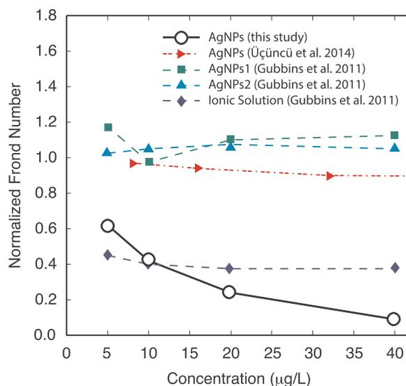
Fig. 3. Reduction of *Lemna minor* frond number when the toxicity tests are conducted with AgNPs produced by spark ablation in the gas phase (this study), AgNPs produced by classical wet-chemistry methods (Gubbins et al., 2011), AgNPs produced by laser ablation in the liquid phase (Üçüncü et al., 2014), or Ag ionic solutions (Gubbins et al., 2011).
