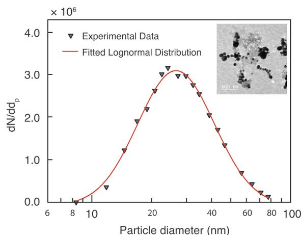
Fig. 2. Size distribution of the test AgNPs measured by the apparatus shown in route 1 of Fig. 1. Inset: Scanning Electron Microscope images of particles collected on a microscopy grid.
