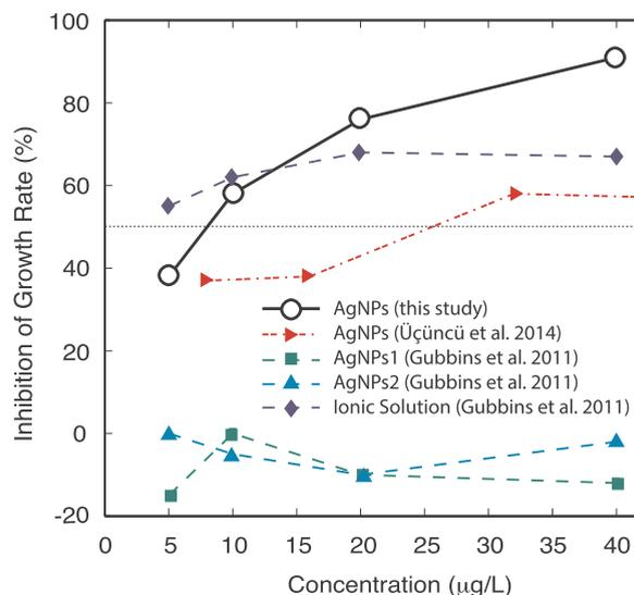
Fig. 4. Inhibition of Growth Rate (%) of *Lemna minor* frond number when exposed to AgNPs produced by spark ablation (black line with black circles; this study), AgNPs produced by classical wet-chemistry methods (green and red lines with diamonds and triangles corresponding to different particle sizes; Gubbins et al., 2011) AgNPs produced by laser ablation in the liquid phase (red line with triangles; Üçüncü et al., 2014), and ionic silver (blue line with diamonds; Gubbins et al., 2011).
