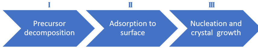
Figure 2.6.: Schematic of the three basic steps of graphene formation.
