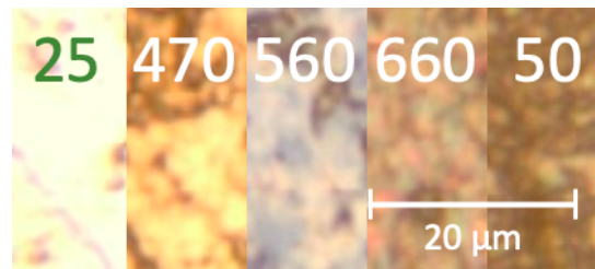
Figure 4.8.: Optical micrographs of the 1.5 μm nickel coating at different temperatures in air. The colours appear analogous to those on pure Ni.
