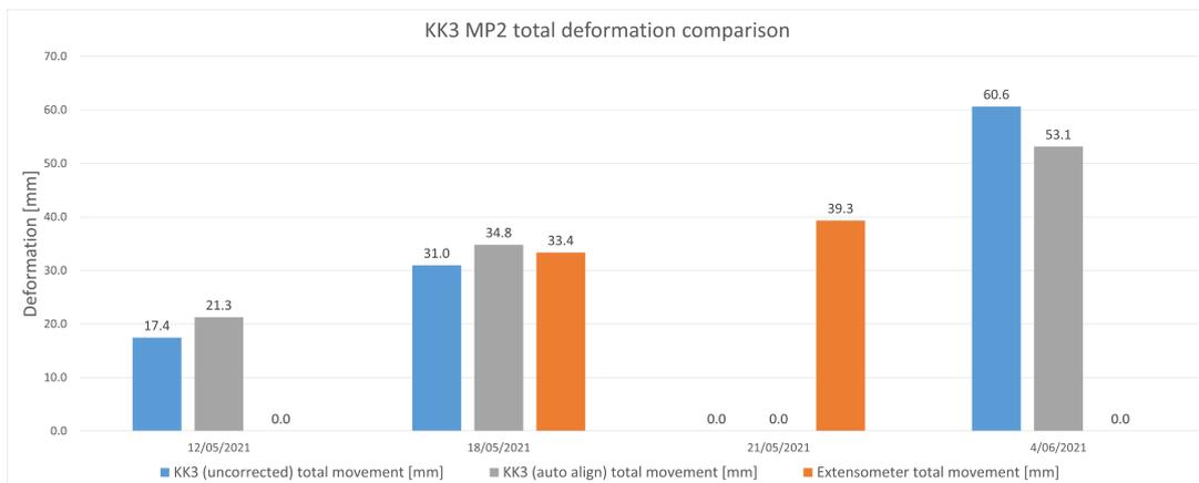
Figure 6.50: Comparison of LiDAR total deformation results vs tape extensometer results at KK3 location 1, measurement point 2.
