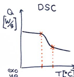
Figure 3.2: Schematic representation of a DSC measurement in the 'exo up' mode to get positive heat flow rates for exothermic processes. Here only part of the second second heating ramp is shown that contains the step with onset and endset points, which mark the  $T_g$  range, indicated in orange
