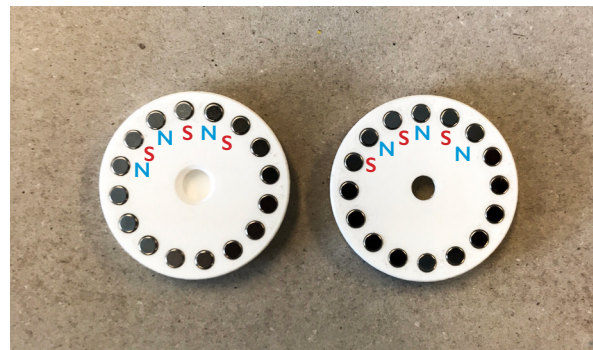
Figure 49: Magnetic drive discs, with pole indication
