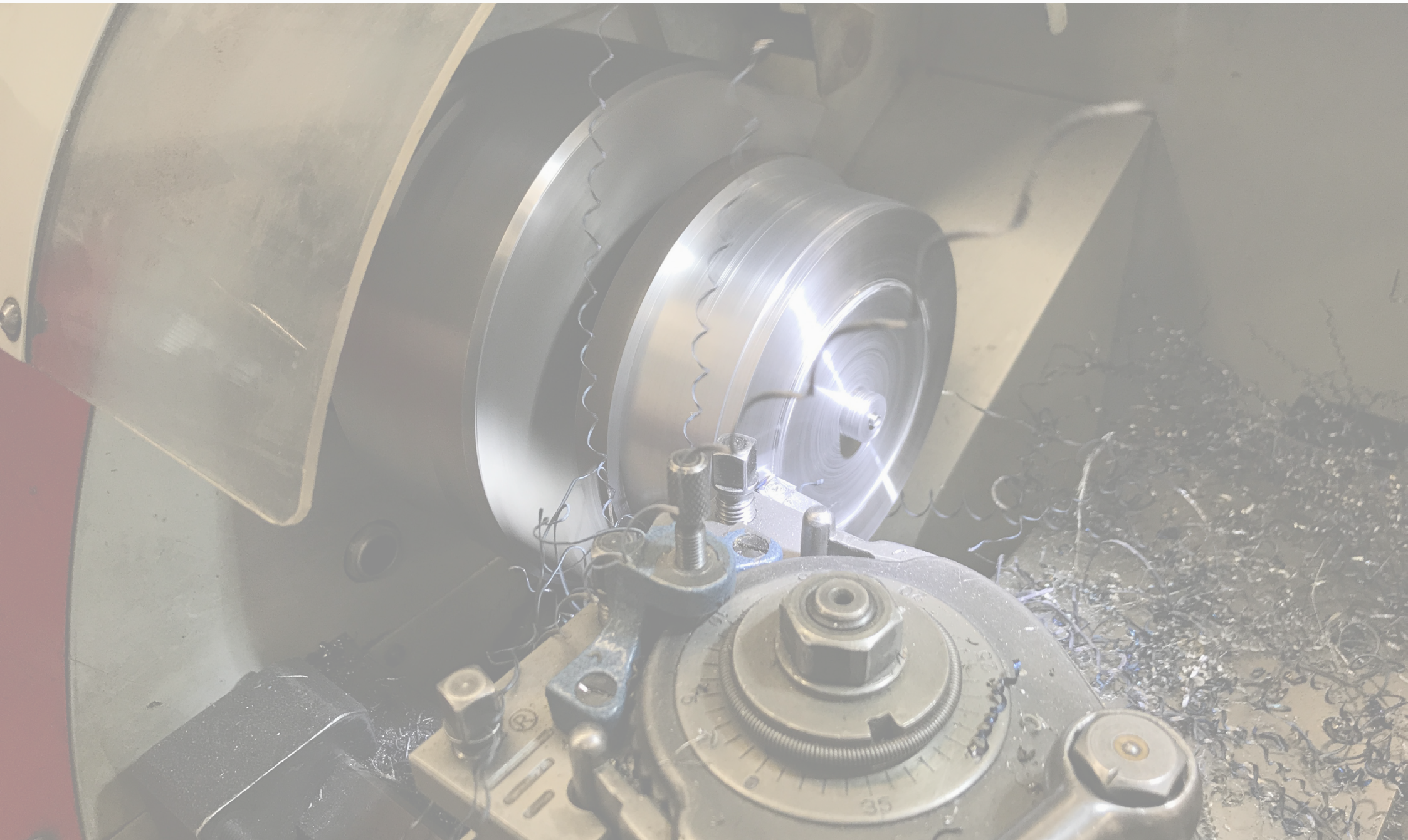
Figure 29: Embodiment in progress; a prototype flywheel rotor is being lathed.
