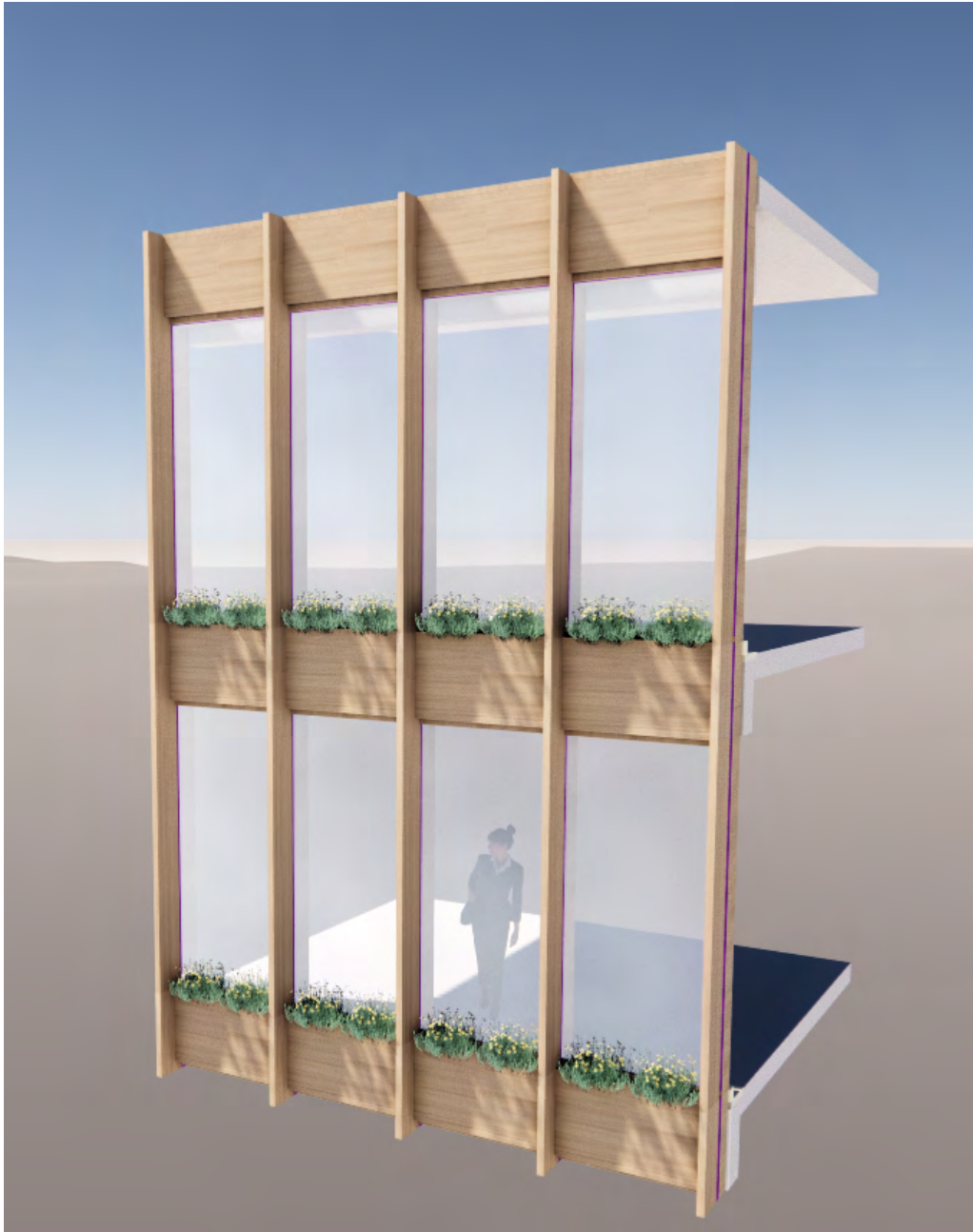
Render 11: Composite Timber Facade fragment. Author's own work.
