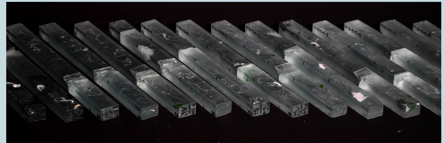
Figure 96: Experiment Type 2: Composite beams, focus on the optimal ratio between surface and bulk
