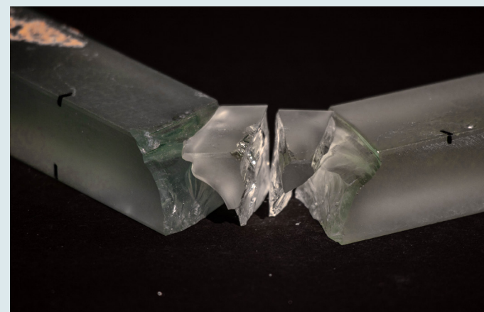
Figure 100: Beam with a high energy failure. This is a composite beam
