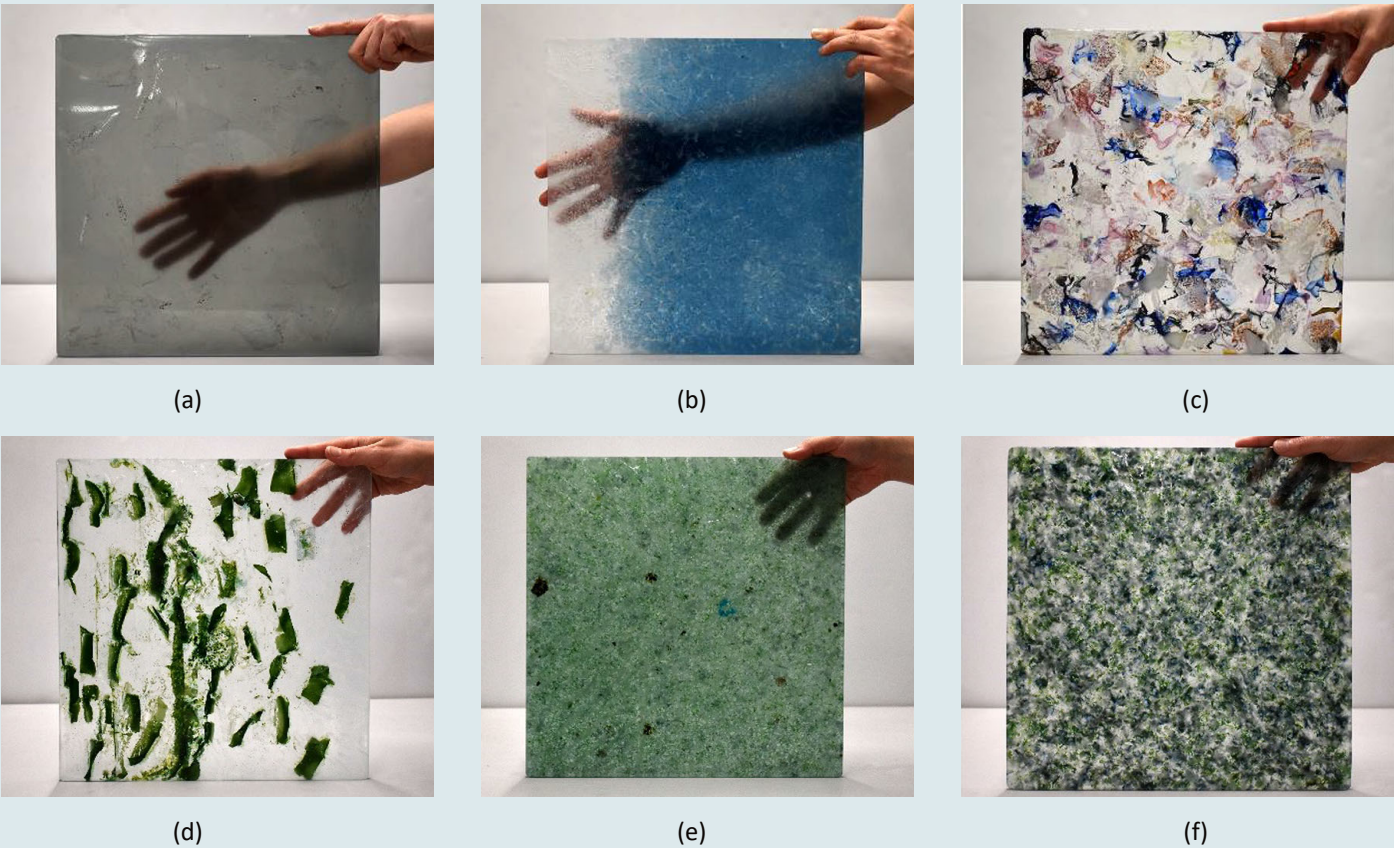
Figure 36: (a) Glass kiln-cast panels (350*350*10 mm) made at TU Delft from glass waste cullet, namely Cathode-Ray Tube (CRT) front screen, (b) transition Float glass from clear to blue, (c) CRT back screen and crystal coloured glass, (d) enamel Float glass, (e) automotive glass and (f) oven doors. (Bristogianni & Oikonomopoulou, 2023)
