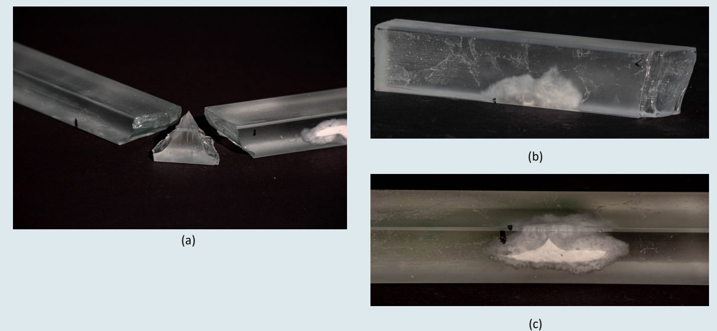
Figure 110: Inclusion in a composite beam in the bulk, Beam V-2B-C8-C-3 (a) location of the crack, (b) side view and (c) front view
