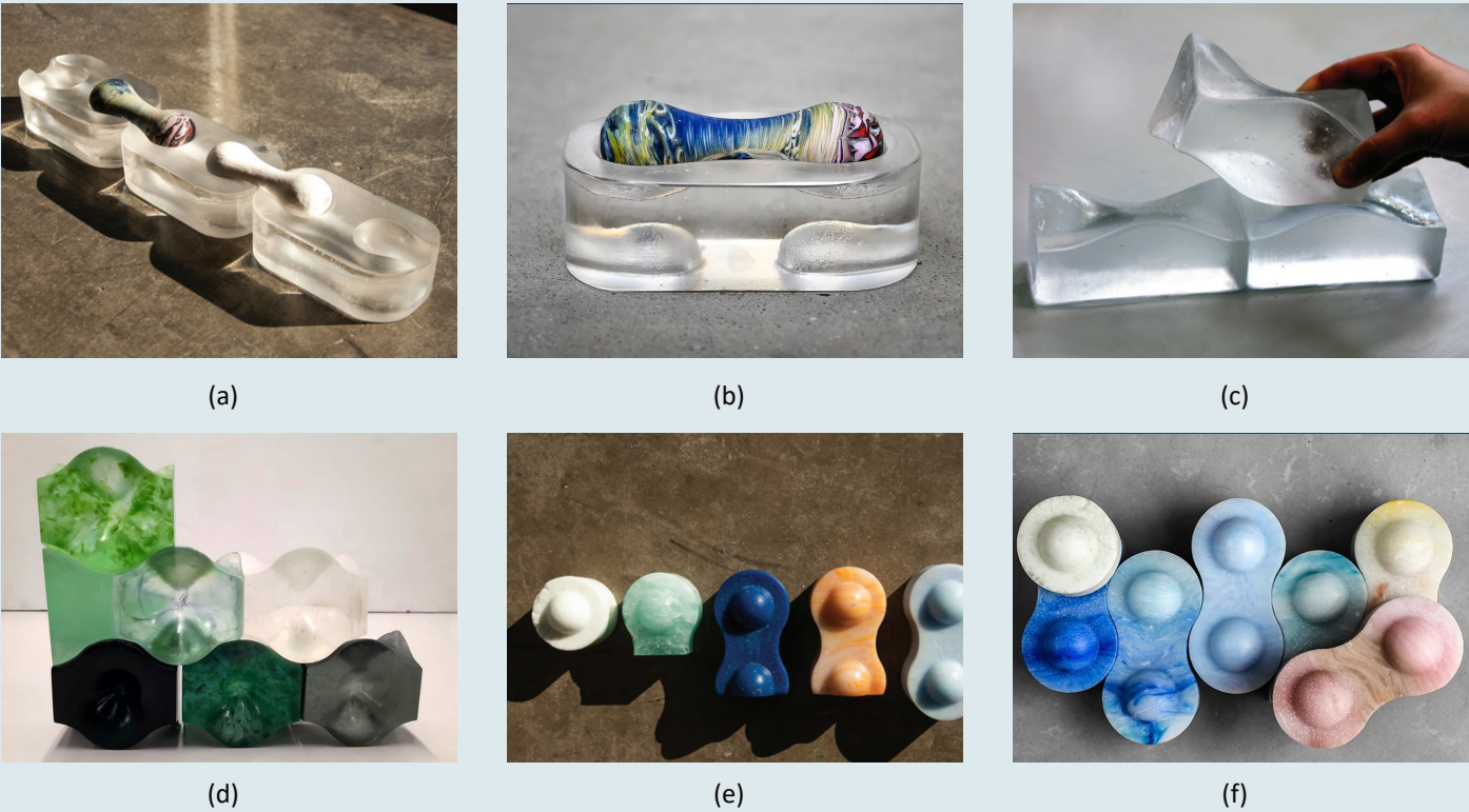
Figure 37: (a) Interlocking waste glass component, (b) Interlocking waste glass component, (c) Structural cast glass components out of different glass waste streams, to be used in an interlocking wall system, (d) Structural cast glass components out of different glass waste streams, to be used in an interlocking wall system, (e) Re3 casted component and (f) Re3 casted component. (Restruct TU Delft, 2024)
