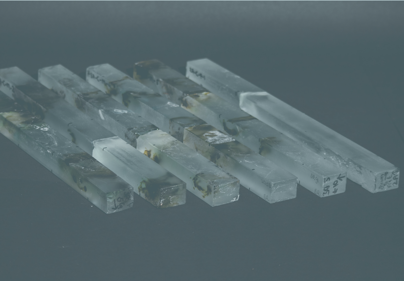
Figure 93: Experiment Type 3: Composite beams, focus on influence of the material composition of the bulk
