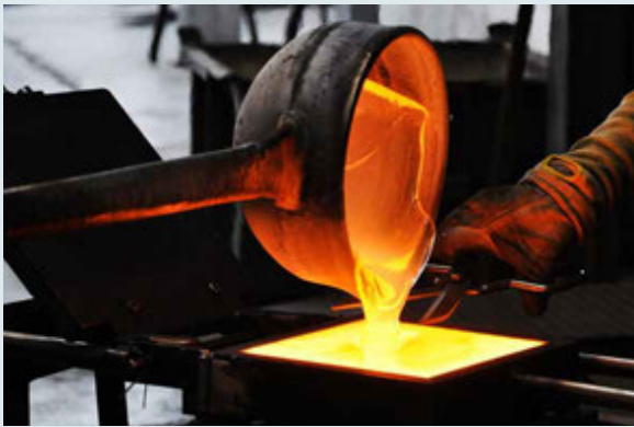
Figure 14: Casting of soda-lime glass blocks at Poesia Factory in Italy. (Oikonomopoulou, 2019)
