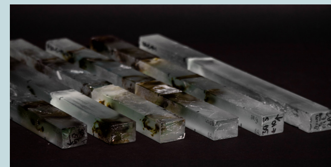
Figure 97: Experiment Type 3: Composite beams, focus on influence of the material composition of the bulk
