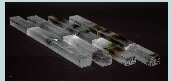
Figure 98: Experiment Type 4: Composite beams, focus on influence of the material composition of the surface
