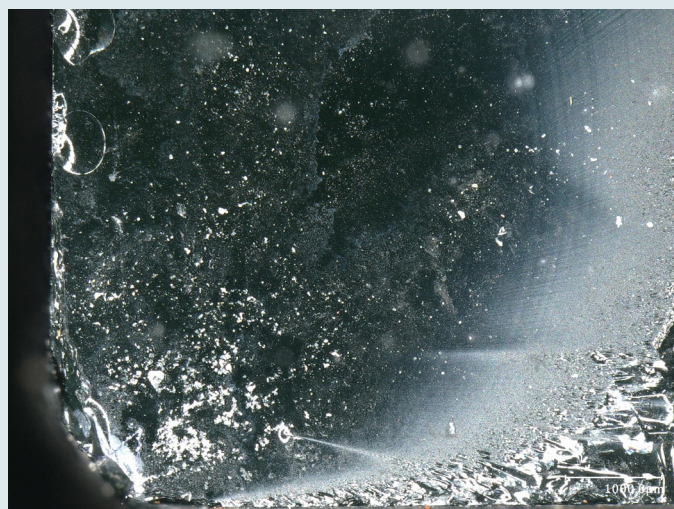
Figure 103: Beam with a low energy failure. A big mirror located at the fracture. This is a composite beam with Fritted glass.
