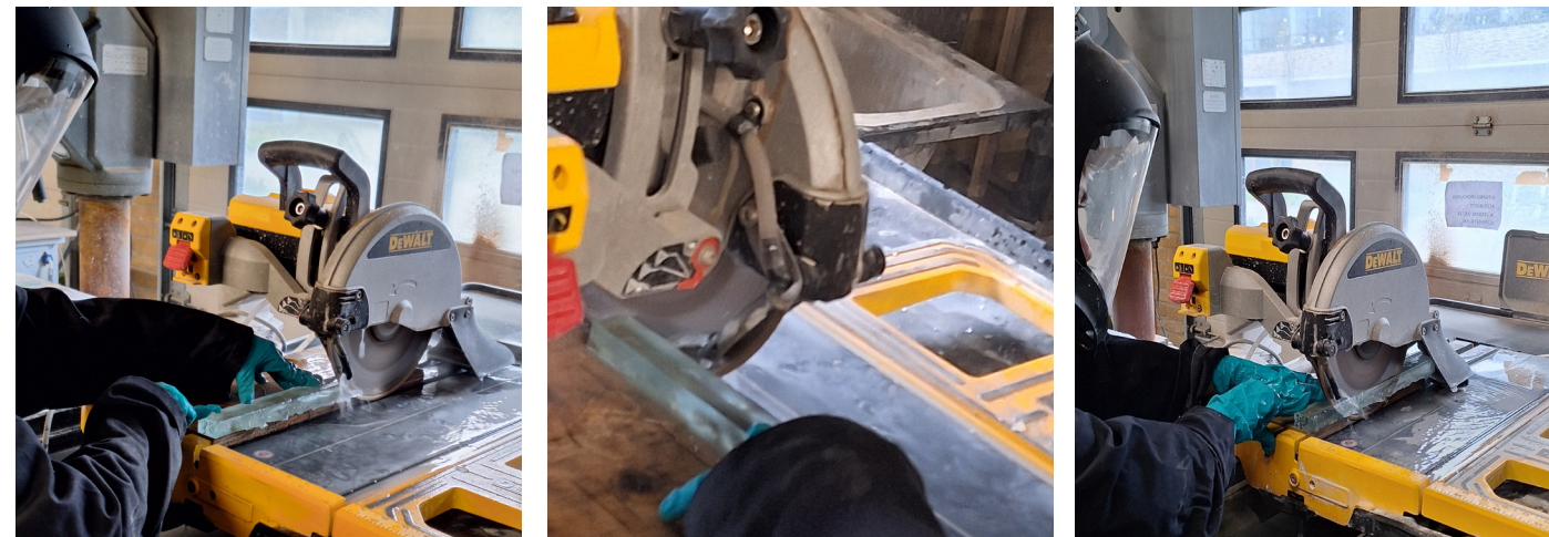
Figure 86: Cutting the beams with a diamond saw
