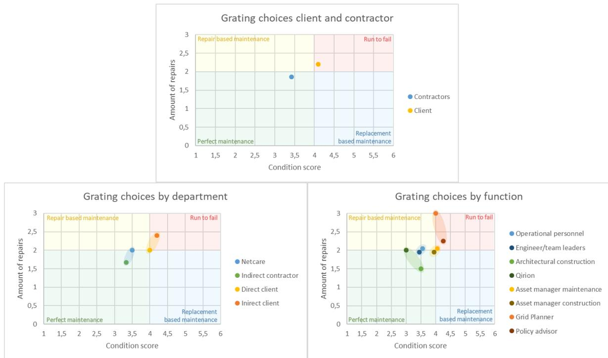
Figure 7-16: Condition and repair choices for the grating
