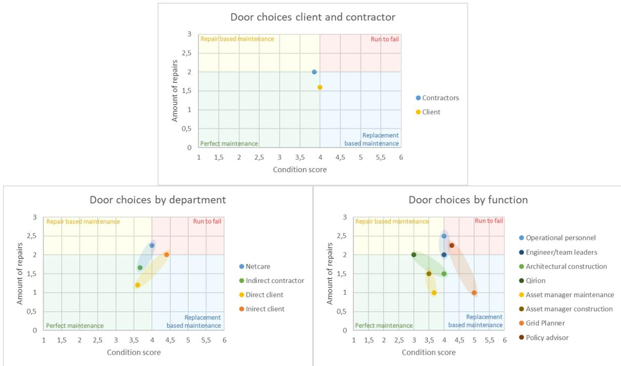
Figure 7-12: Condition and repair choices for the door
