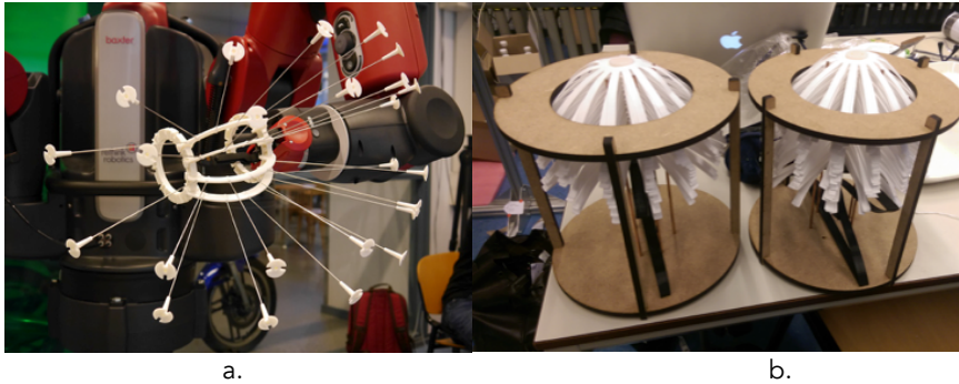
Figure 33 (a) Petal ribs assembled onto the top assembly; (b) Two petal dispensers.
