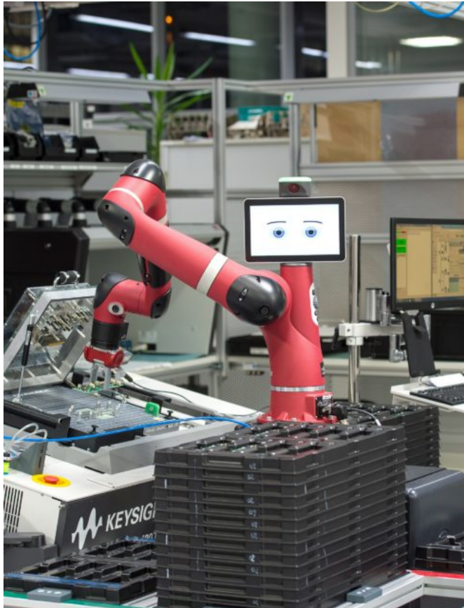
Figure 2 A Collaborative Robot in action. (Rethink Robotics, Sawyer) (Image copyright ©Rethink Robotics)
