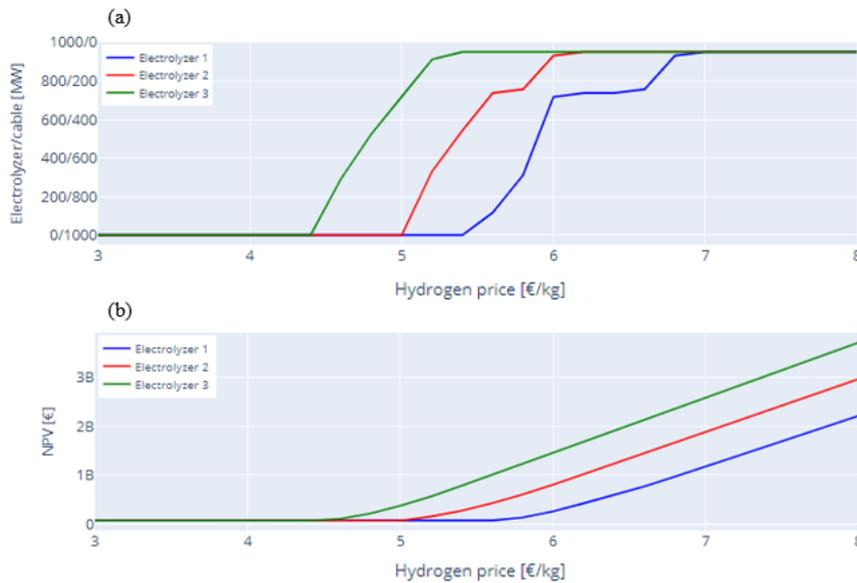
Figure 4.13: Results of the scenario analysis with a mean electricity price of €75 per MWh. In Figure (a), the optimal EC ratio as a function of the hydrogen price is presented. The corresponding NPV is found in Figure (b).
