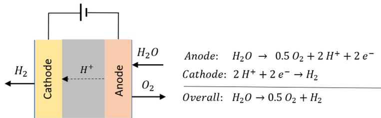
Figure 2.5: The PEM electrolyzer process with the half-reactions occurring at the electrodes
