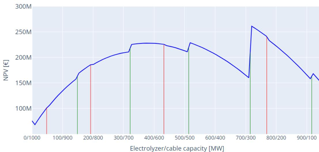
Figure 4.3: NPV as a function of connection ratio. The total connection size adds up to the total capacity of the wind farm (1000MW).
