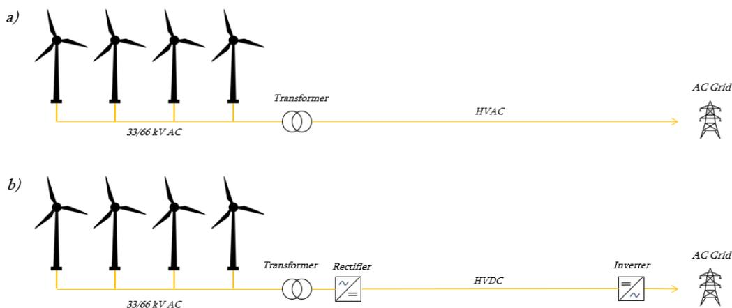
Figure 2.8: Simplified design of a) a HVAC transmission line and b) a HVDC transmission line.
