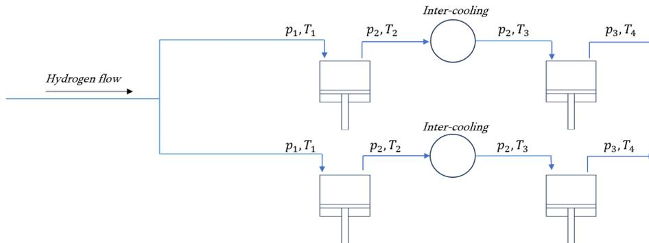
Figure 3.3: Schematic example of the reciprocating piston compressor system. In this example, the hydrogen flow is distributed over two compressor stations with inter-cooling devices.
