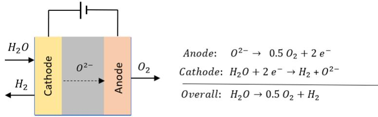
Figure 2.6: The SOE process with the half-reactions occurring at the electrodes
