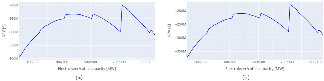
Figure 4.6: Results of the sensitivity analysis on the wind farm costs. Figure (a) illustrates the NPV for a scenario with -15% cost of wind energy, and Figure (b) shows the NPV for a scenario with a wind farm that is 15% more expensive.
