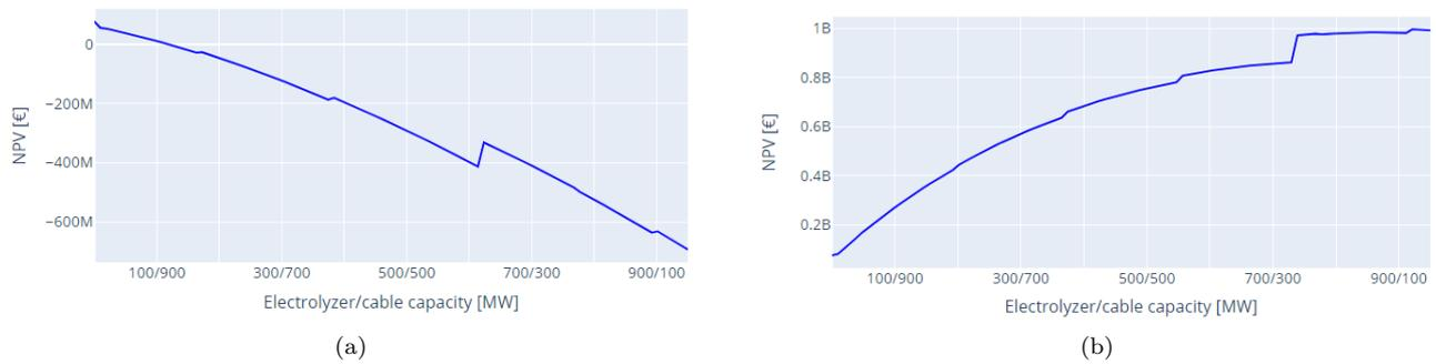
Figure 4.9: Results of the sensitivity analysis on the electrolyzer efficiency. Figure (a) depicts the NPV for a scenario with a  $-15\%$  efficiency, and Figure (b) presents the NPV for a scenario with a  $+15\%$  efficiency.
