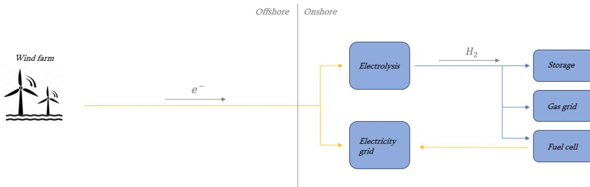
Figure 1.2: Overview of a hybrid wind farm using onshore electrolysis.
