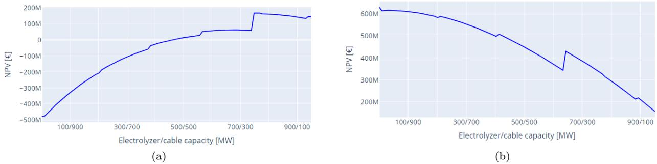
Figure 4.11: Results of the sensitivity analysis on the mean electricity price. Figure (a) presents the NPV for a scenario with a 15% decline in electricity price, and figure (b) shows the NPV for a scenario with a cost of electricity that is 15% higher.
