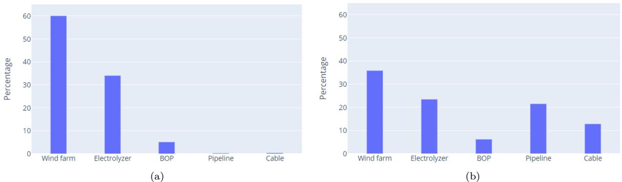
Figure 4.4: Economic analysis per system component. In Figure (a), the share of each component to the total CAPEX is depicted. Figure (b) presents the percentage of the components to the total OPEX.
