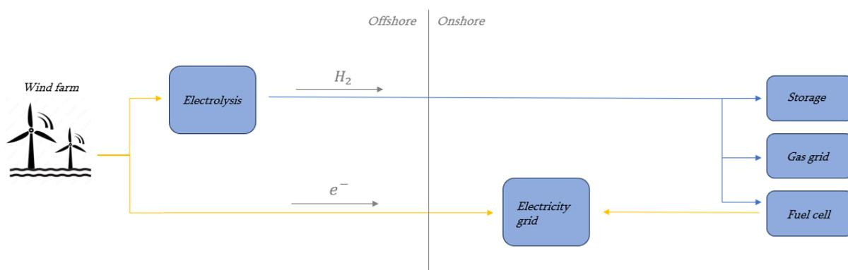
Figure 1.3: Overview of a hybrid wind farm using offshore electrolysis.
