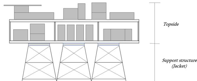
Figure 2.2: Schematic representation of an offshore platform with a jacket support structure.
