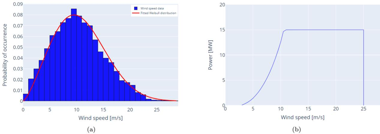
Figure 3.1: Wind farm specifications with (a) a histogram of used wind speed data with in red the fitted Weibull distribution. The Weibull distribution has a scale parameter  $c$  of 12.05 and a shape parameter  $k$  of 2.35. And (b) the power curve of the considered 15 MW wind turbine.
