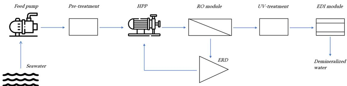
Figure 2.3: Schematic representation of the proposed water treatment system.
