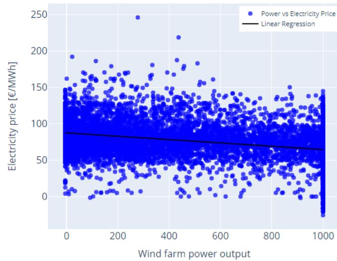
Figure J.3: Electricity price against wind farm power output. The black line indicates the correlation between the two.
