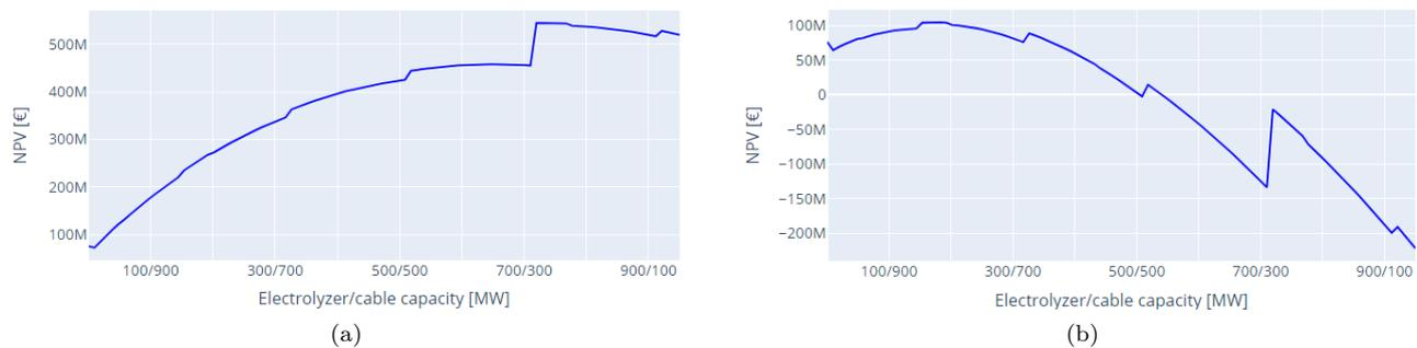
Figure 4.7: Results of the sensitivity analysis on the electrolyzer cost. Figure (a) illustrates the NPV for a scenario with a 15% cost reduction, and Figure (b) shows the NPV for a scenario with a 15% cost increase.
