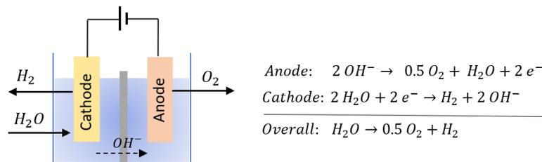
Figure 2.4: The AWE process with the half-reactions occurring at the electrodes.
