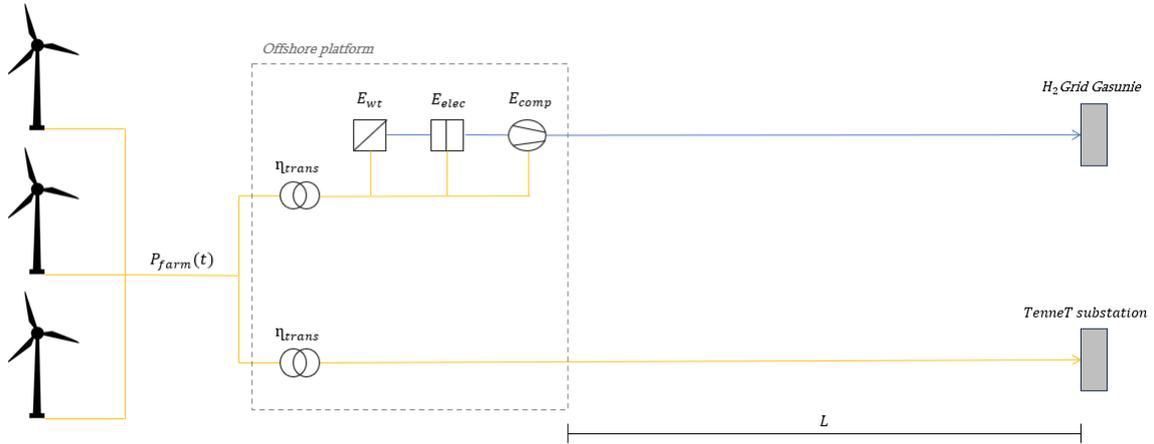
Figure 3.4: Schematic overview of the proposed system. The yellow lines represent the electricity path, and the blue lines indicate the hydrogen path.
