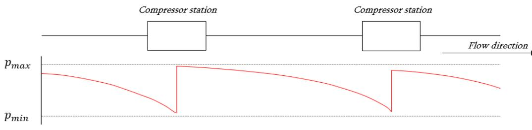
Figure 2.7: The use of multiple compressor stations to maintain the pressure within certain boundaries.
