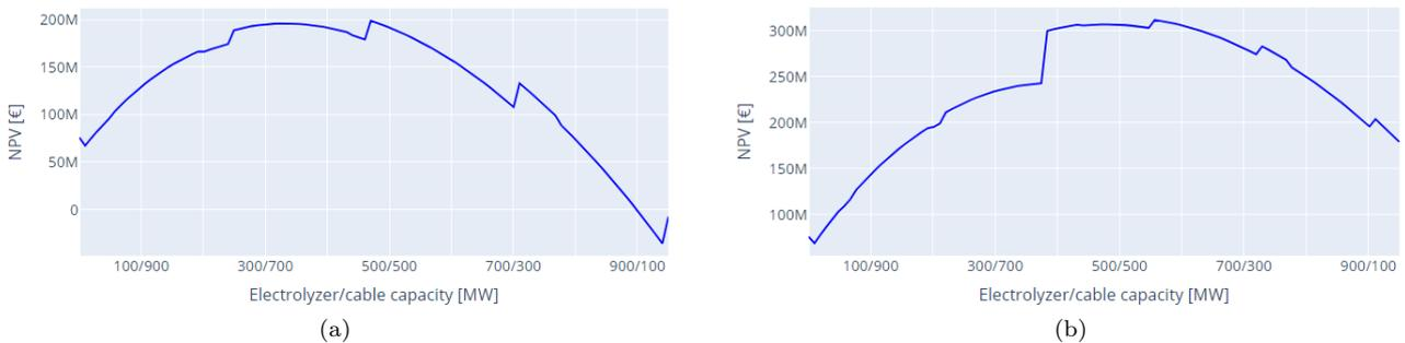
Figure 4.8: Results of the sensitivity analysis on the stack lifetime. Figure (a) illustrates the NPV for a scenario with a 15% lifetime reduction, and Figure (b) shows the NPV for a scenario with a 15% lifetime increase.
