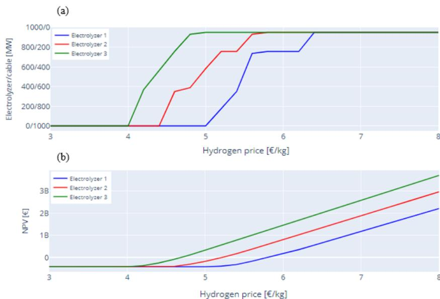
Figure 4.12: Results of the scenario analysis with a mean electricity price of €65 per MWh. In Figure (a), the optimal EC ratio as a function of the hydrogen price is presented. The corresponding NPV is found in Figure (b).
