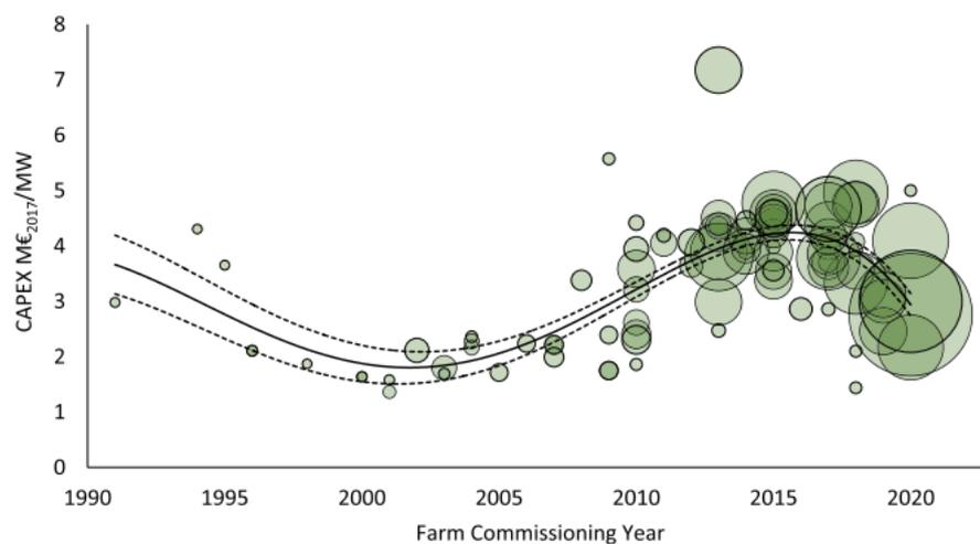
Figure E.2: Specific cost in M€/MW for offshore windfarms from 1991 to 2020. A 4th-order polynomial fit is included within the margins for its 95% confidence interval. The graph was taken from Viera et al. [61].
