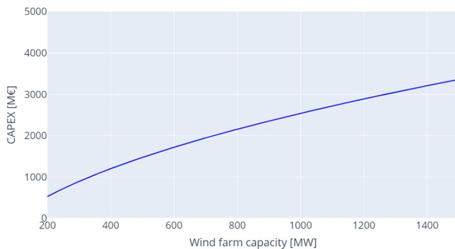
Figure E.1: Offshore wind farm CAPEX as a function of total farm capacity. This curve is based on historical data [61] and holds for a water depth of 30 meters and a turbine capacity of 15 MW
