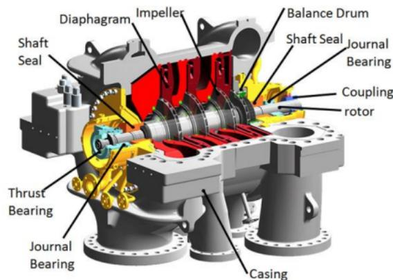
Figure 2.10: Schema of a centrifugal compressor [57].
