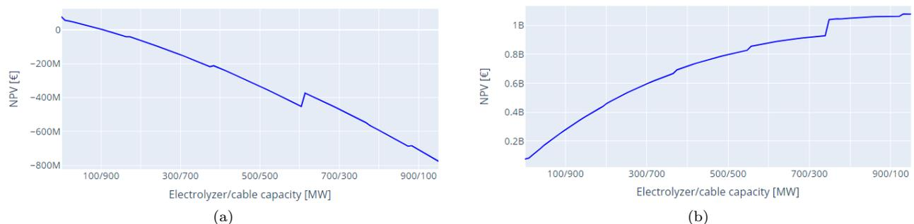
Figure 4.10: Results of the sensitivity analysis on the hydrogen price. Figure (a) illustrates the NPV for a scenario where the hydrogen price is decreased by 15%, and figure (b) shows the NPV for a scenario with a cost of hydrogen that is 15% higher.
