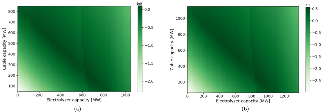
Figure 4.5: Results of the sensitivity analysis on the capacity of the wind farm. Figure (a) illustrates the NPV for a farm with 850 MW capacity, and Figure (b) shows the NPV for an 1150 MW wind farm.
