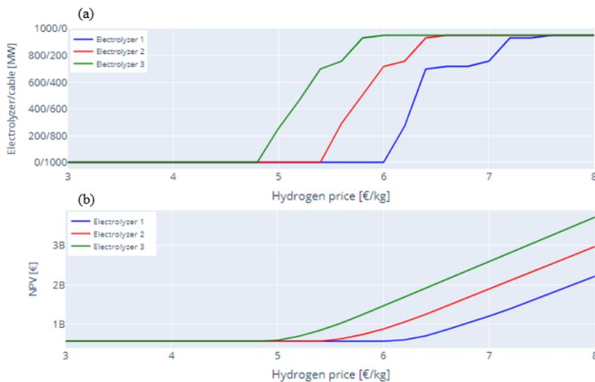
Figure 4.14: Results of the scenario analysis with a mean electricity price of €85 per MWh. In Figure (a), the optimal EC ratio as a function of the hydrogen price is presented. The corresponding NPV is found in Figure (b).
