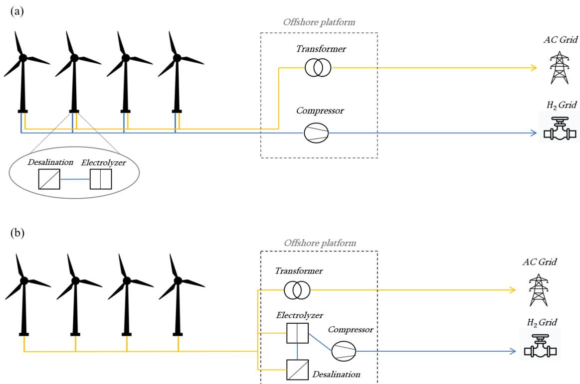
Figure 2.1: Two hybrid wind farm concepts proposed by the literature. With (a) representing the 'in-turbine' configuration and (b) the 'centralized' concept.
