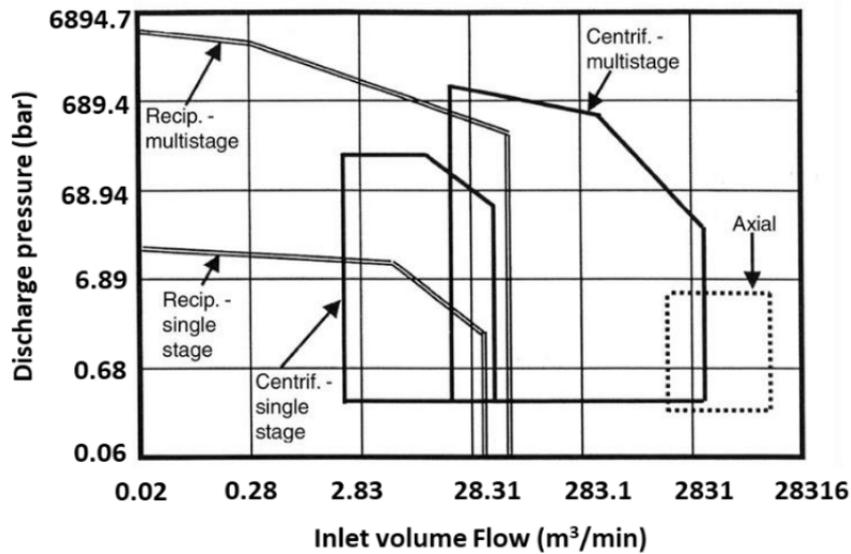
Figure I.1: Diagram for compressor selection. The diagram was adopted from [57].
