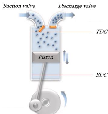
Figure 2.9: Schema of a reciprocating compressor [57].
