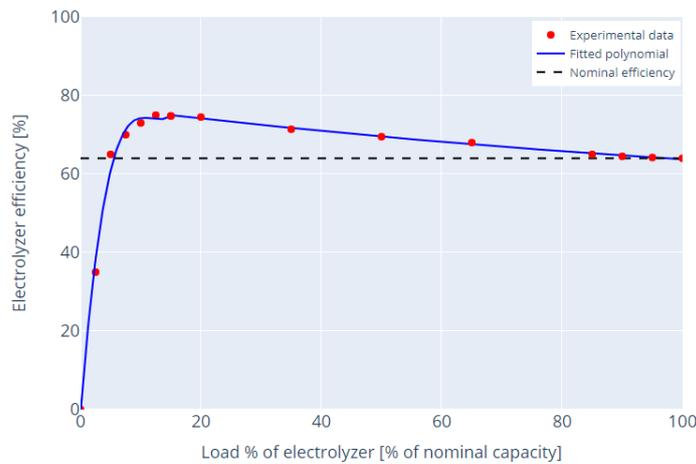
Figure 3.2: PEM electrolyzer efficiency based on load percentage relative to its nominal capacity. The experimental data was taken from Kopp et al. [68]
