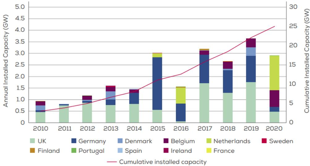
Figure 1.1: Annual installed offshore wind capacity in Europe. The line represents the cumulative installed capacity [1].
