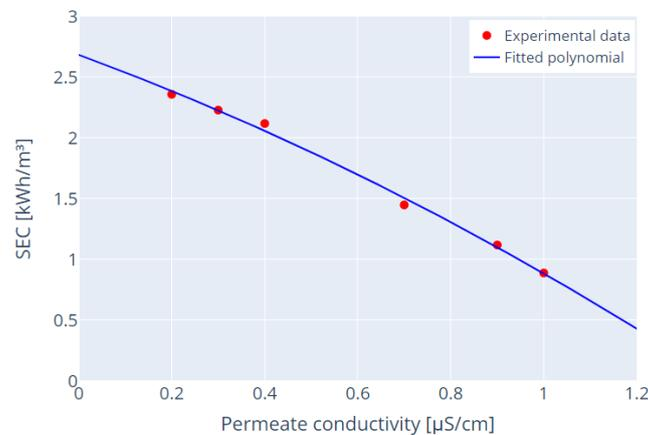
Figure F.2: SEC of deionizing tapwater ( $248 \mu\text{S}/\text{cm}$ ) for various permeate conductivities. Experimental data were taken from Warandi et al. [64]. A 2nd-order polynomial was fitted through their data points:  $y = -0.395x^2 - 1.404x + 2.684$
