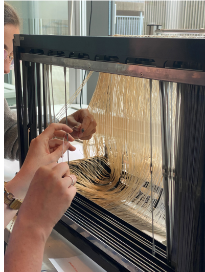
Figure 1.6: Each yarn of the warp has to pass through one head of the correspondent shaft (see Figure 1.2)
