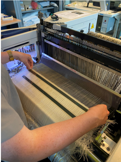
Figure 1.11: Weaving of weft can finally begin, in the case of Suntext the solar panels are added manually
