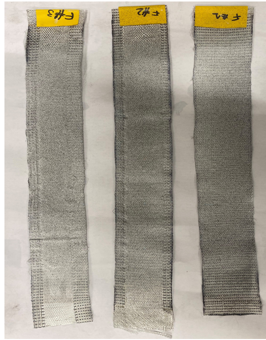
Figure 3.20: Weft (or fill) specimens after the application of a speckle patterned necessary for DIC system
