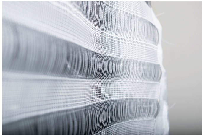
Figure 1.1: A woven solar integrated textile currently under development [Pauline van Dongen Studio]
