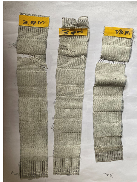
Figure 3.45: Warp specimens after testing. From left W03, W02, W01.
