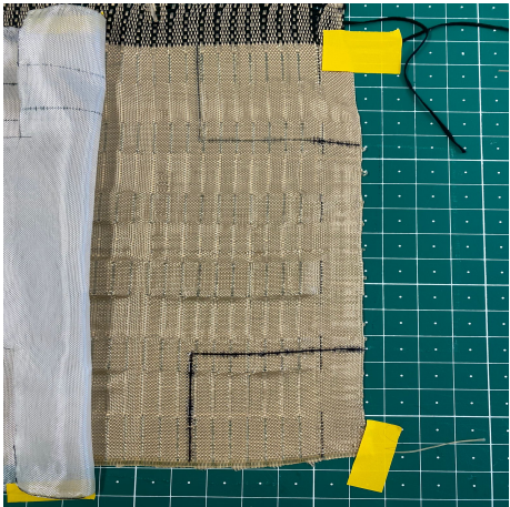
Figure 3.14: The geometry follows the yarn pattern making perpendicular angles
