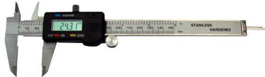
Figure 3.71: Caliper used to measure deformation
