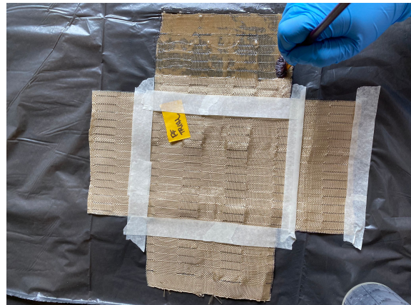
Figure 3.24: The same comparison of two different types of glue has been done on the picture frame trial specimen (hand woven)
