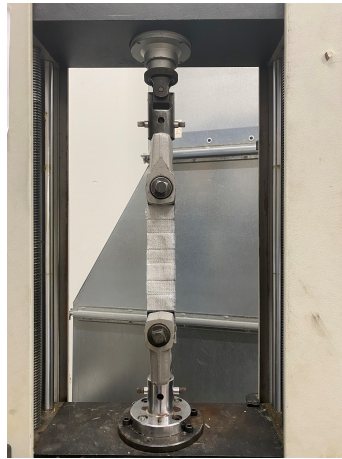
Figure B.1: Tensile machine test set up (W01: Warp is aligned with tensile extension)
