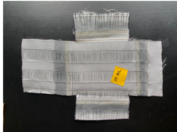
Figure 3.26: On the Suntex specimens only the latex-based glue was used. Specimen PF1 before punching the holes.
