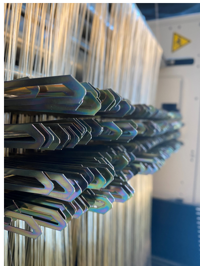
Figure 1.10: The height of the warp droppers represents the tension along each yarn
