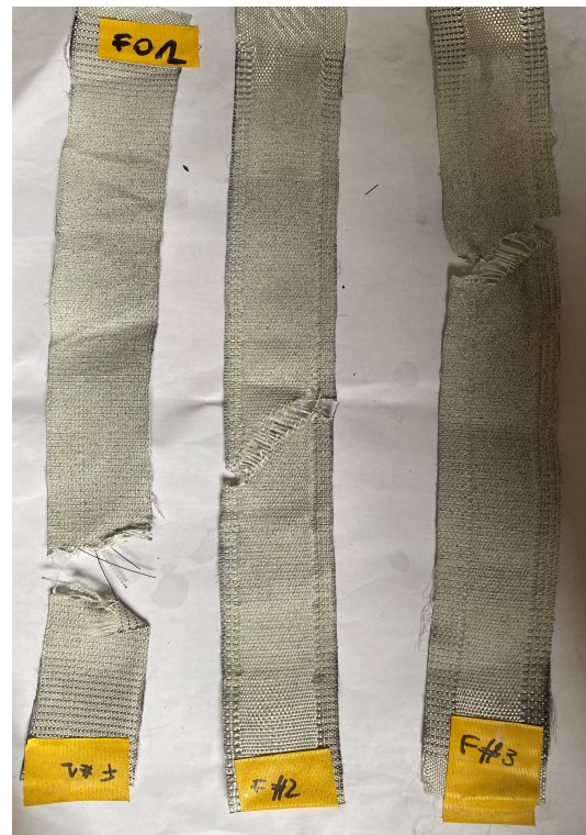
Figure B.29: Weft specimens after testing. From left F01, F02, F03.
