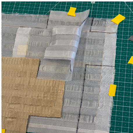
Figure 3.17: The geometry follows the yarn pattern making perpendicular angles
