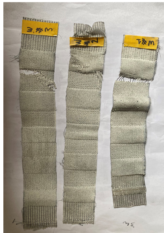
Figure B.15: Warp specimens after testing. From left W03, W02, W01.
