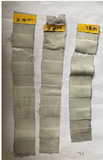
Figure 5.1: Warp specimens after testing. From left W03, W02, W01.
