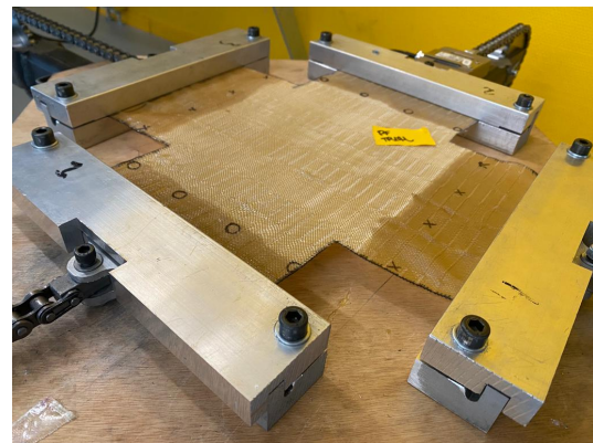
Figure 3.53: Specimen after pre-tension on bi-axial ring
