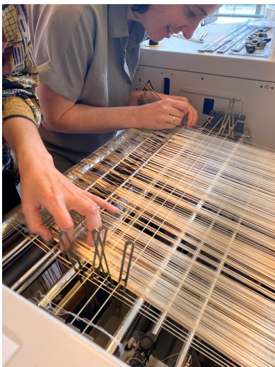
Figure 1.9: Here the warp droppers need to be applied to each yarn
