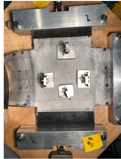
Figure 3.77: extension of flange failure on EL02 specimen
