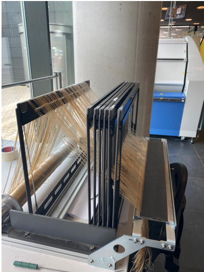
Figure 1.7: They have then to pass through the beater (or reed), this process is also done manually
