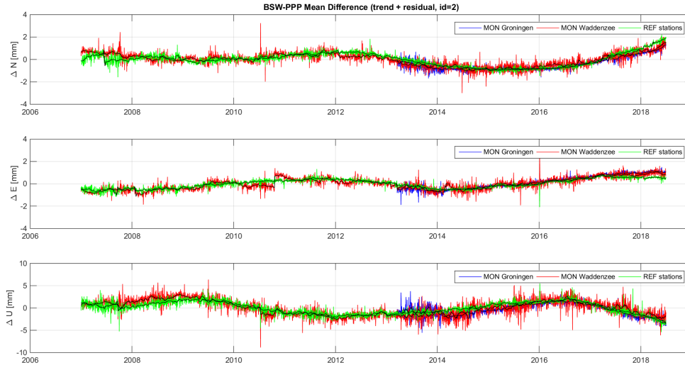
Figure 7.3: Average trend differences between the BSW and PPP solutions for the NAM monitoring and reference stations for the period 2007.0 - 2018.6 : SUM_TREND+RESIDUAL_BSW-PPP . The colored lines are time series of daily averages for respectively the NAM monitoring stations in the Groningen area, monitoring stations in the Waddenzee area and the NAM reference stations. The black lines are the moving 21 day median of the daily averages (with outlier and step detection).
