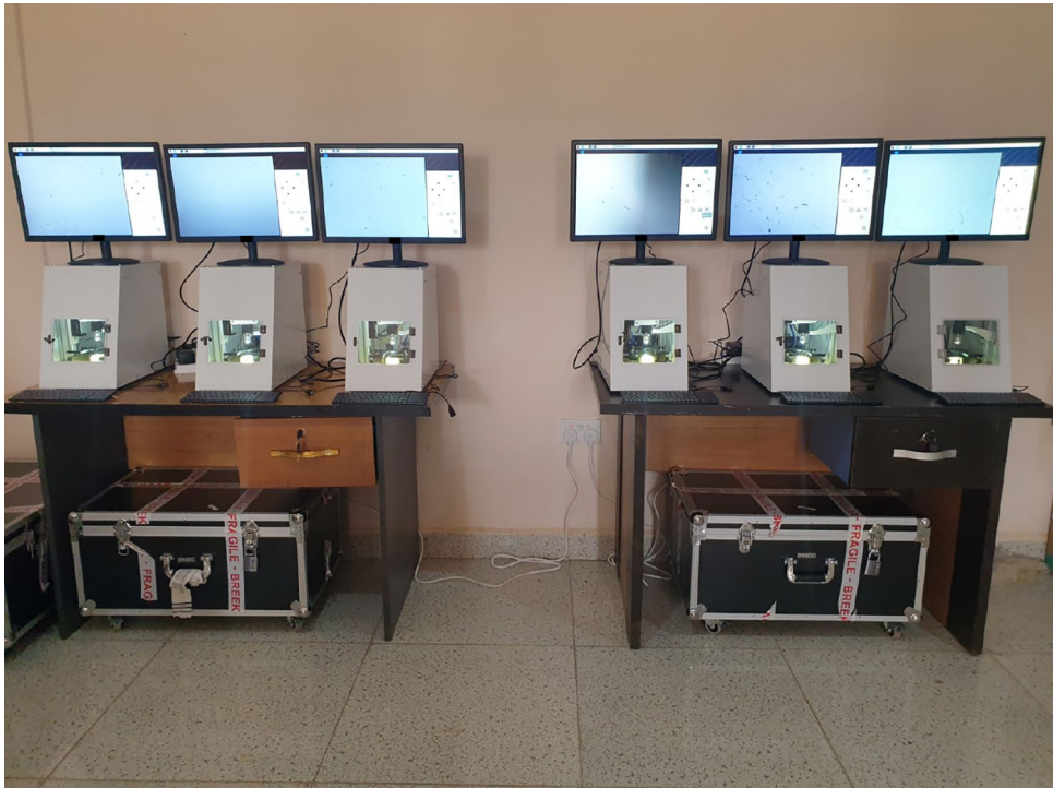
Fig. 1. Field laboratory setup, equipped with 6 Schistoscope devices.
