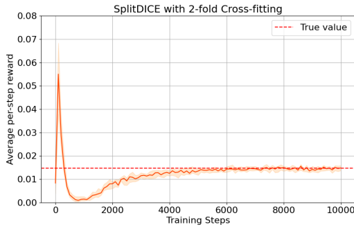
(b) The sample data is split into two distinct subsets at random, namely training and evaluation. Then, the roles of the two datasets are reversed for the second fitting. The final estimate value is calculated as the average of the two fittings.
