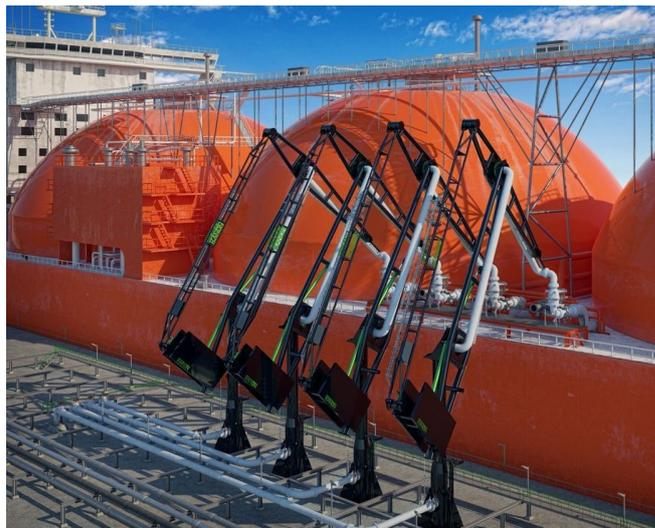
Figure 6.1: Cargo loading arm structure, image from [8]
