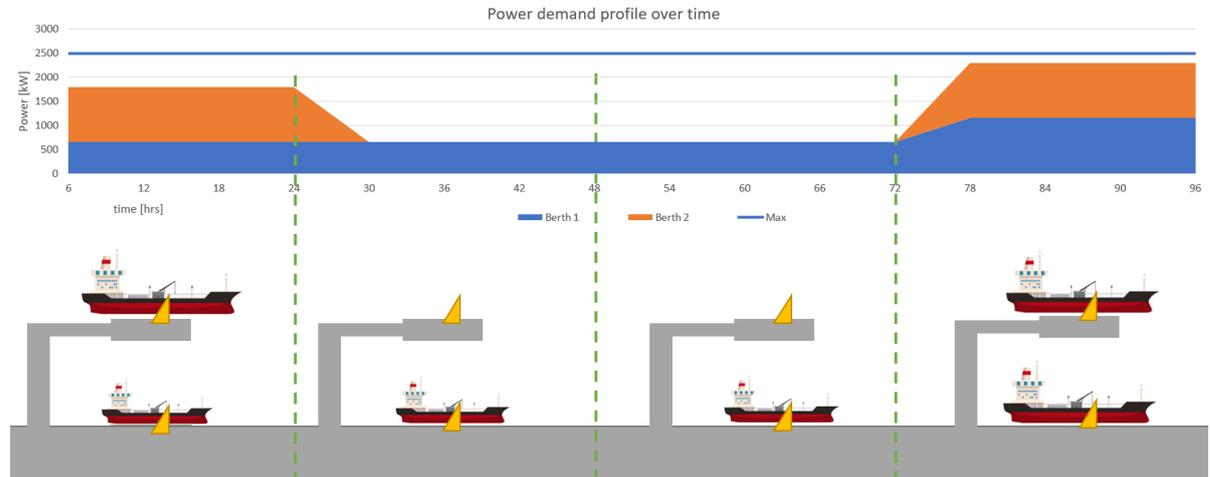
Figure 7.5: The simplified average power demand illustrated over 4 days, with each day different vessels in size and numbers (own figure)
