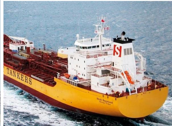
Figure 8.2: A 44,000 dwt chemical vessel, where the aftship is slightly more spacious.
