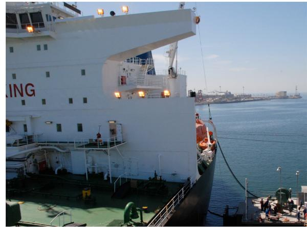
Figure 6.3: Aft - shore cable reel, the crane lifts the cables towards the onboard cable tray [10]
