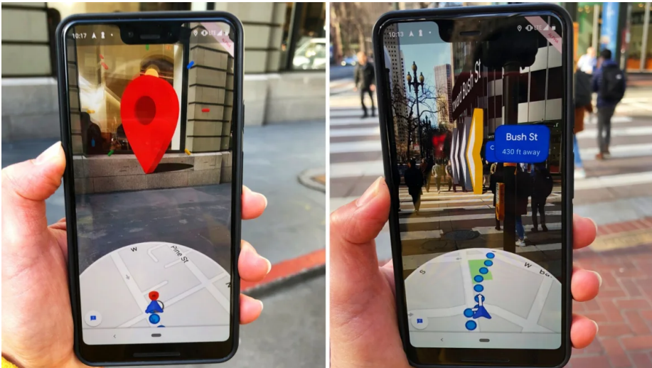
Figure 1.1: An exemplar application of accurate localization is the latest advances in Google Maps. A live camera feed is used to accurately localize the phone’s position and orientation, formally the 6 Degrees-of-Freedom (6-DoF) pose, with respect to a map. This pose then enables augmenting the image with useful navigational guidance.
