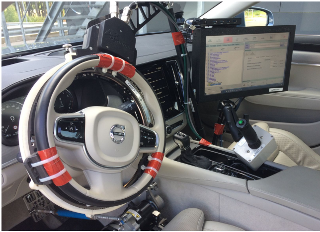
Fig. 9: Steering robot used for executing driving trajectories.
