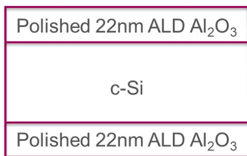
Figure 4-1 Schematic of the double side mirror polished sample, 22nm Al<sub>2</sub>O<sub>3</sub> was deposited on the low-doped n-type c-Si bulk by ALD process
