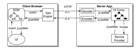
Fig. 1. Processing View of a SPIAR-based architecture.
