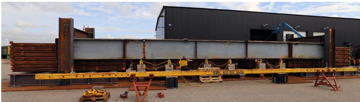
Figure 5 – Trial testing of rig used as verification- and acceptance of the method before full-scale bridge testing
