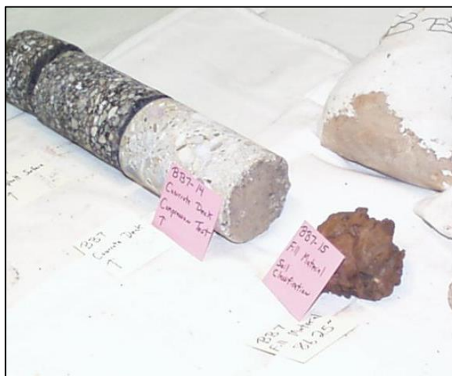
Figure 2 — Sample Core Extracted from the Barnett Bridge
