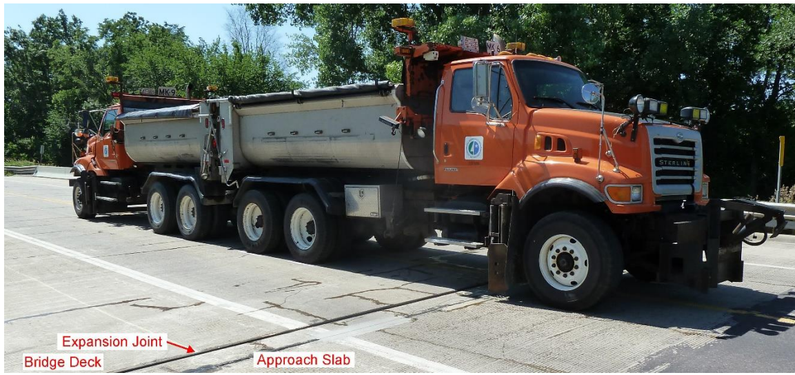
Fig. 1—Back-to-back trucks positioned to maximize live load shear in the smallest rear tandem axle footprint
