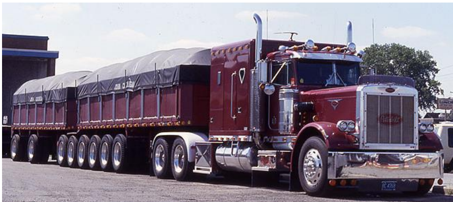
Figure 4 Michigan Truck Train #8 – 134-kip (596 kN) supplementary design load
