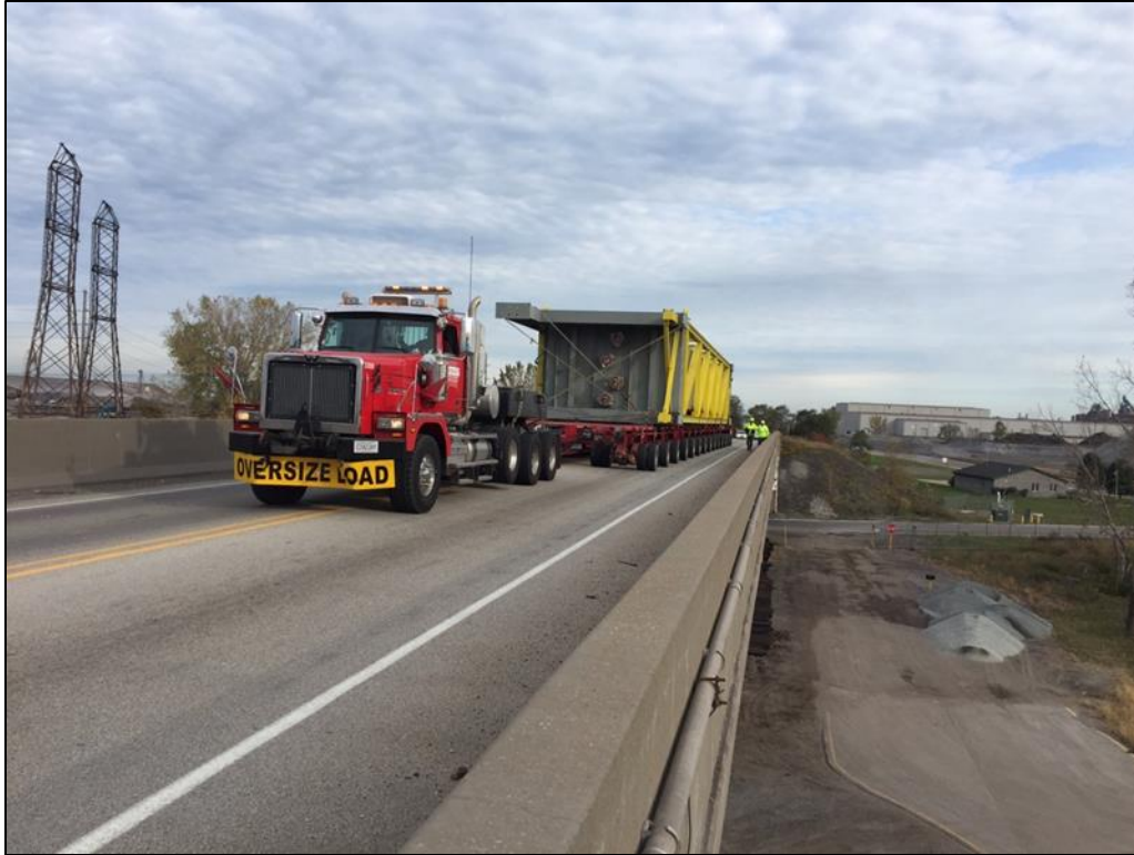
Figure 18 Super-heavy permit vehicle crossing Burns Harbor Bridge -Module A 848-kip (3770 kN)
