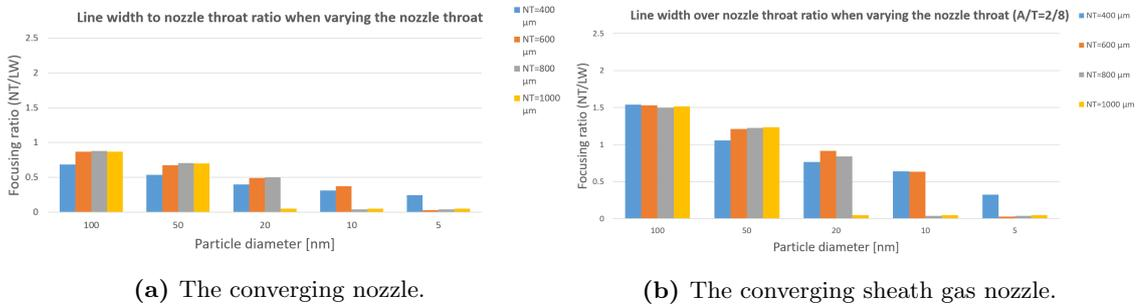
**Figure 4.8:** The focusing ratios (nozzle exit throat/line width) of different particle sizes when changing the nozzle exit throat of a converging and converging sheath gas nozzle.
