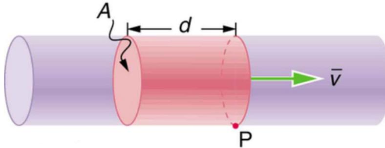
**Figure 3.4:** A fluid channel to illustrate the volumetric flow rate equation. [68]
