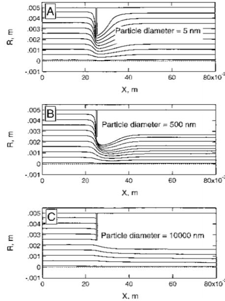
**Figure 2.8:** A schematic representation of the trajectories of different particles sizes through an aerodynamic lens. [22]
