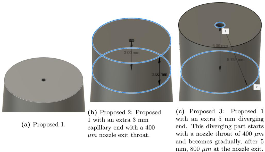
**Figure 5.14:** The differences between the three proposed nozzles.
