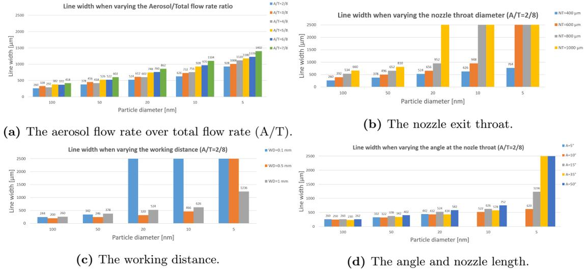
**Figure 4.6:** The line width of different particle sizes when changing different parameters of a converging sheath gas nozzle. Values above 2500 microns indicate that (most of) the particles did not deposit.
