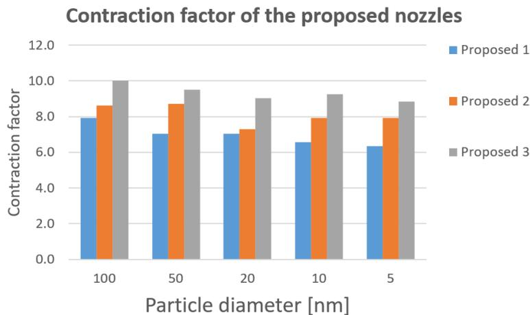
**Figure 5.4:** The contraction factor of different particle sizes of the proposed nozzles.
