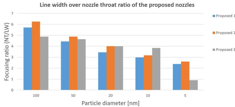
**Figure 5.6:** The focusing ratio (nozzle exit throat/line width) of different particle sizes of the proposed nozzles.
