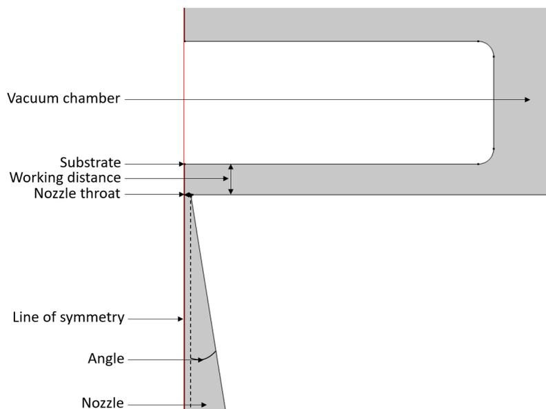
**Figure 3.1:** Graphical explanation of the geometry of a standard (converging) nozzle.
