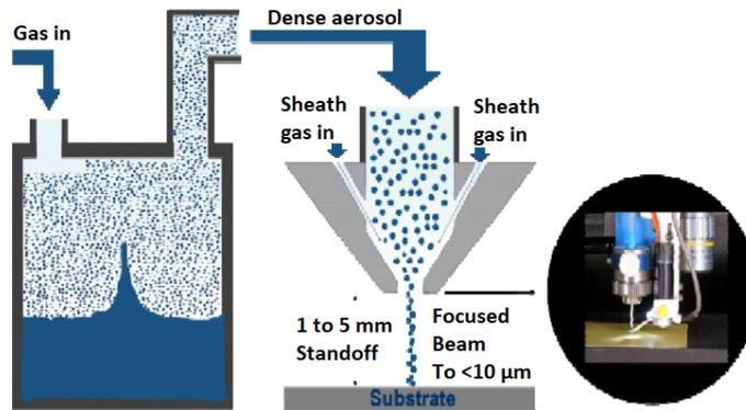
**Figure 1.3:** A schematic representation of the Aerosol Jet Printer made by Optomec. [21]
