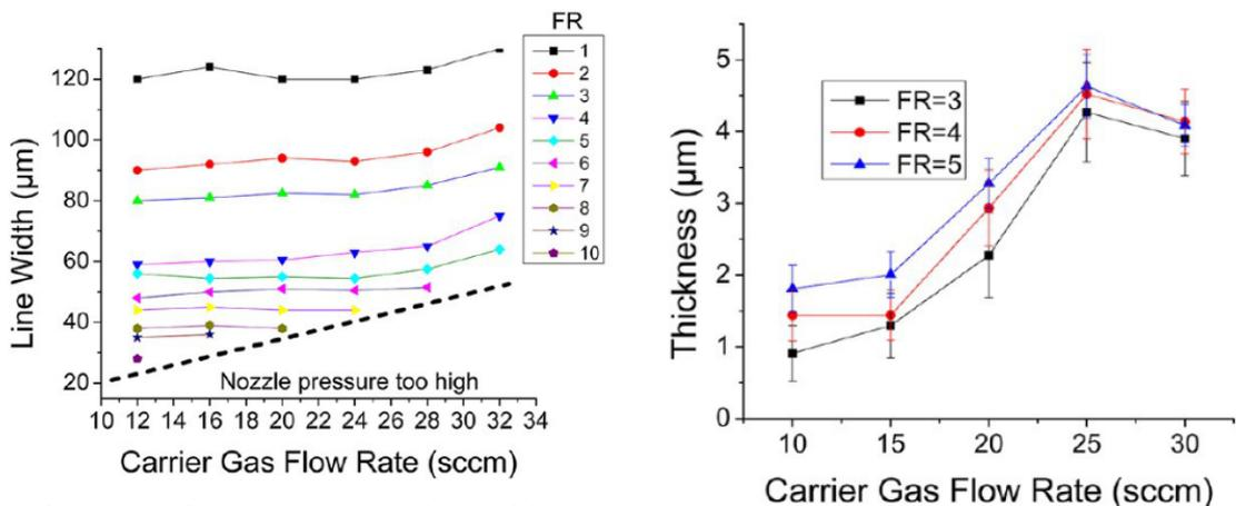
(a) Carrier gas flow rate versus the line width while also considering the focusing ratio.
