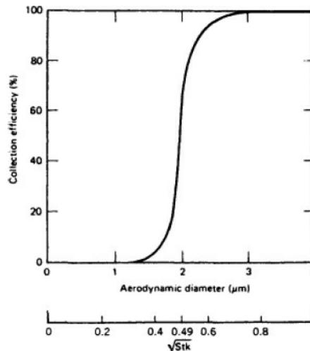
**Figure 2.5:** Impaction efficiency versus particle size. [56]
