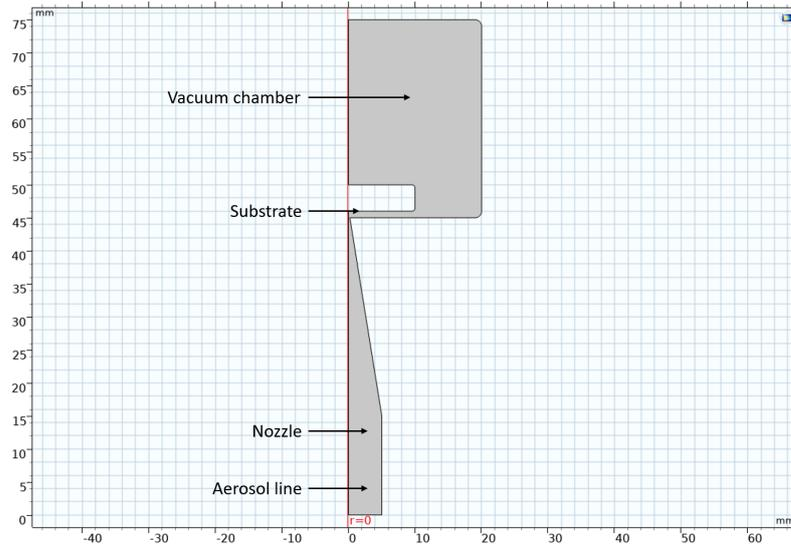
**Figure 3.2:** An example of multiple polygons used to model a standard converging nozzle, substrate and vacuum chamber.
