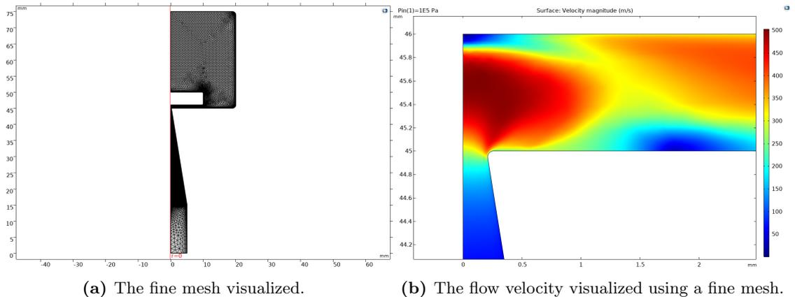
**Figure 3.6:** A fine mesh used to model the flow velocity of a converging nozzle in COMSOL.
