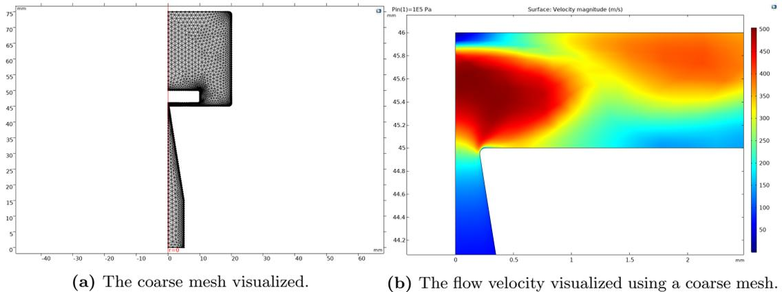
**Figure 3.5:** A coarse mesh used to model the flow velocity of a converging nozzle in COMSOL.
