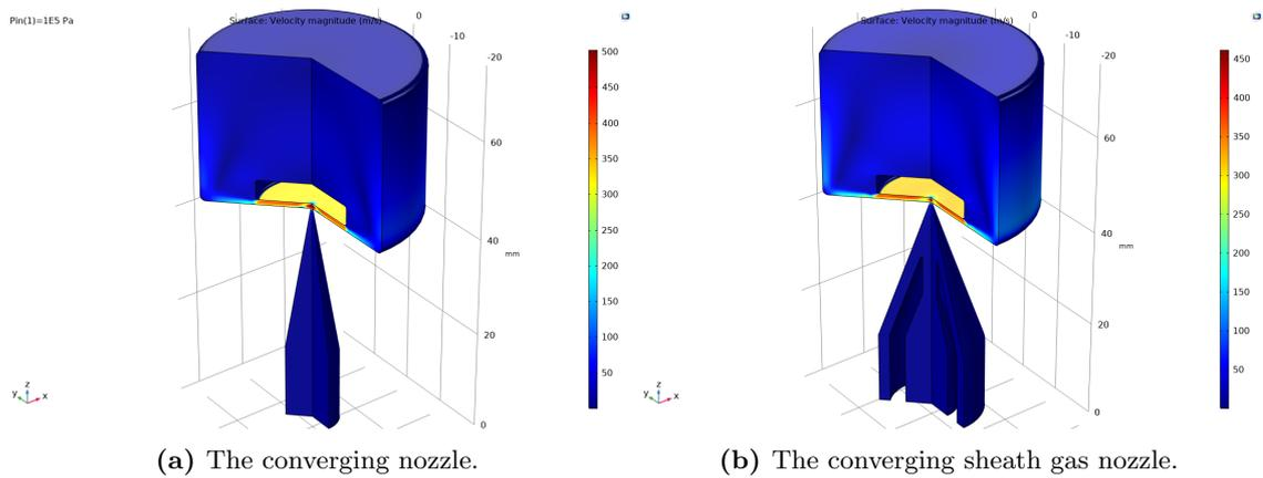
**Figure 3.9:** 3D view of the velocity profiles of the converging and converging sheath gas nozzle.
