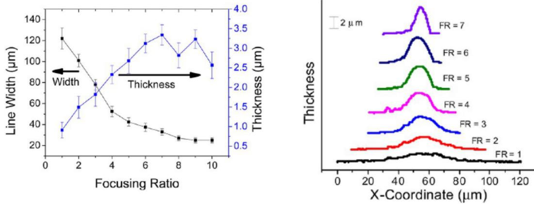
(a) Focusing ratio versus the line width and thickness.
