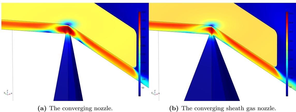
**Figure 3.10:** 3D view of the flow behaviour slightly before and after the nozzle exit throat.
