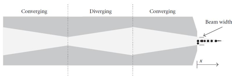
**Figure 2.10:** A schematic representation of a typical converging-diverging-converging nozzle. [63]
