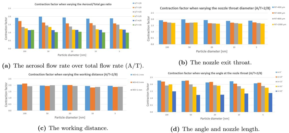
**Figure 4.5:** The contraction factor of different particle sizes when changing different parameters of a converging nozzle.
