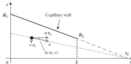
**Figure 2.13:** Radial and axial velocity of the gas in a capillary nozzle implemented with a slightly converging nozzle. [64]
