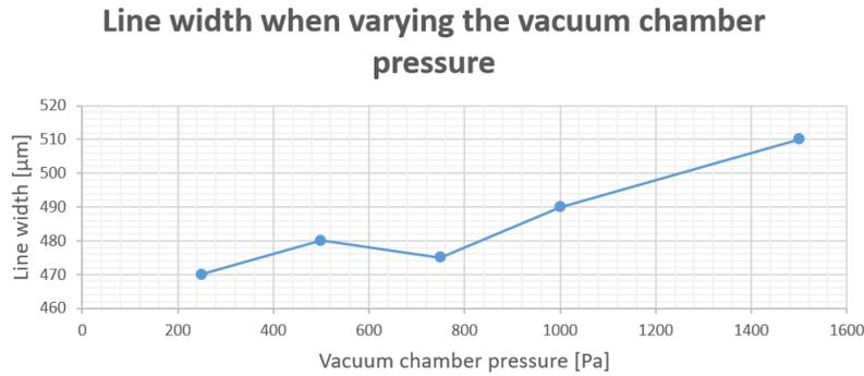
**Figure 5.17:** Line width, using a converging nozzle, when varying the vacuum pressure.
