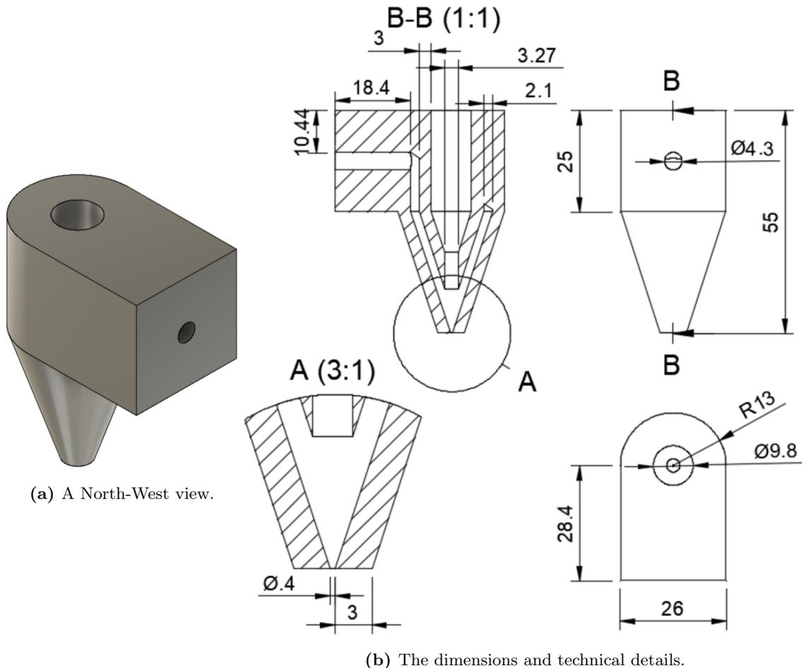
**Figure 5.11:** Modified CAD model of the converging sheath gas nozzle.
