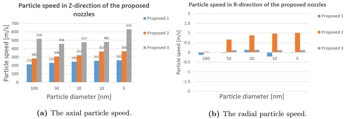
**Figure 5.3:** The particle axial (Z) and radial (R) speeds of different particle sizes of the proposed nozzles. These are the maximum speeds measured at the centerline and exit of the nozzles. The values are interpolated.
