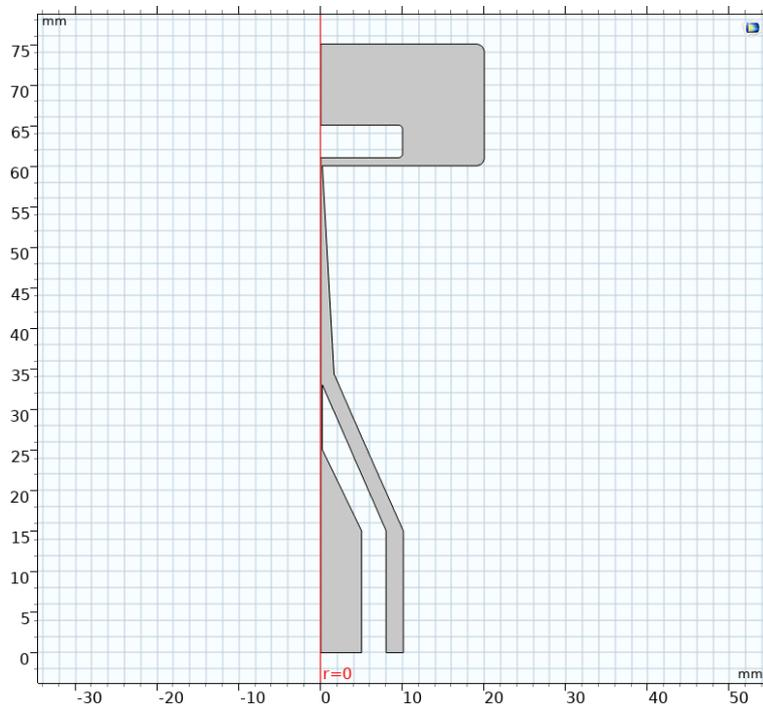
**Figure 5.1:** Proposed converging sheath gas nozzle design.
