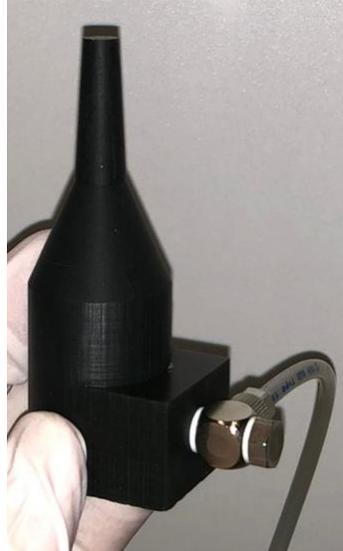
**Figure 5.15:** Proposed 1 connected to the sheath gas line of the SAM setup.
