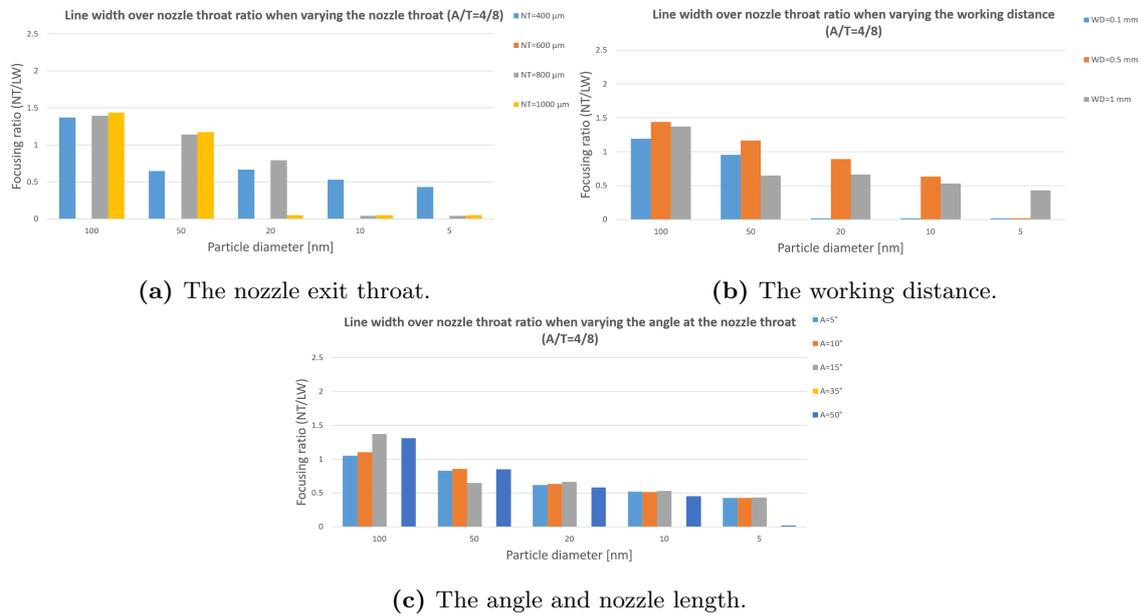
**Figure C.7:** The focusing ratio (nozzle exit throat/line width) of different particle sizes when changing different parameters of a converging sheath gas nozzle with  $A/T=4/8$ .
