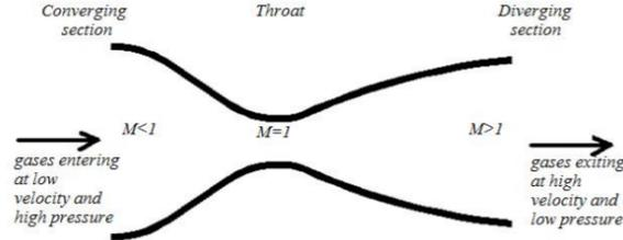
**Figure 2.7:** A schematic representation of an ideal converging-diverging nozzle. [59]
