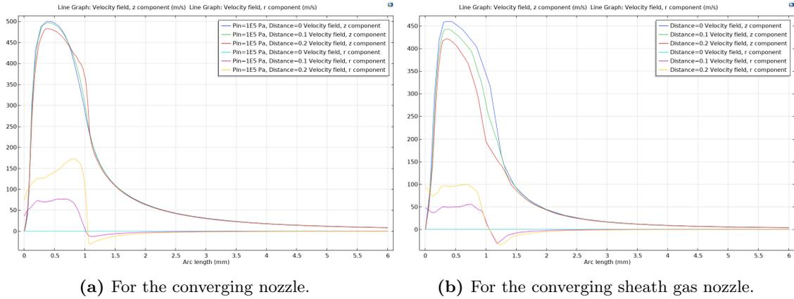
**Figure 3.14:** The z- and r-velocity at different distances from the nozzle axis at the last 6mm before the substrate. The substrate is at 0 mm and the nozzle exit throat at 1 mm, everything after that is in the nozzle.
