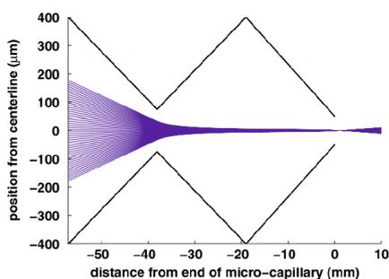
**Figure 2.11:** Collimation of particles in a typical converging-diverging-converging nozzle. [17]
