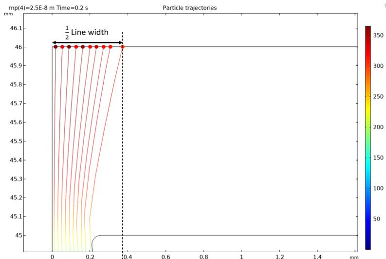
**Figure 3.13:** Converging nozzle used to explain the interpretation of the line width.
