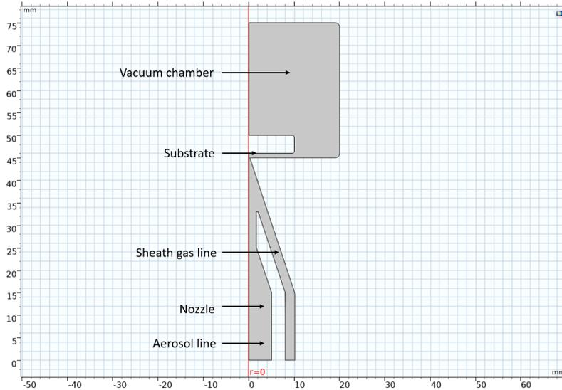
**Figure 3.3:** An example of multiple polygons used to model a converging sheath gas nozzle, substrate and vacuum chamber.
