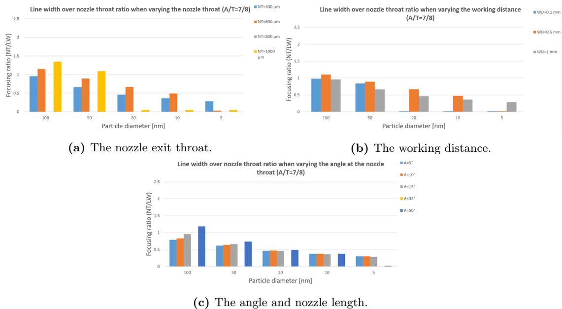
**Figure C.8:** The focusing ratio (nozzle exit throat/line width) of different particle sizes when changing different parameters of a converging sheath gas nozzle with  $A/T=7/8$ .
