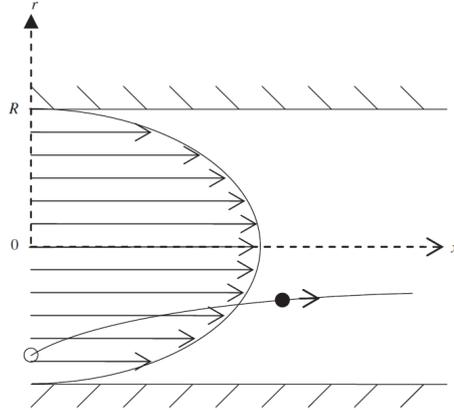
**Figure 2.12:** A schematic representation of the working principle of a capillary nozzle made by Akhatov et al. [64].
