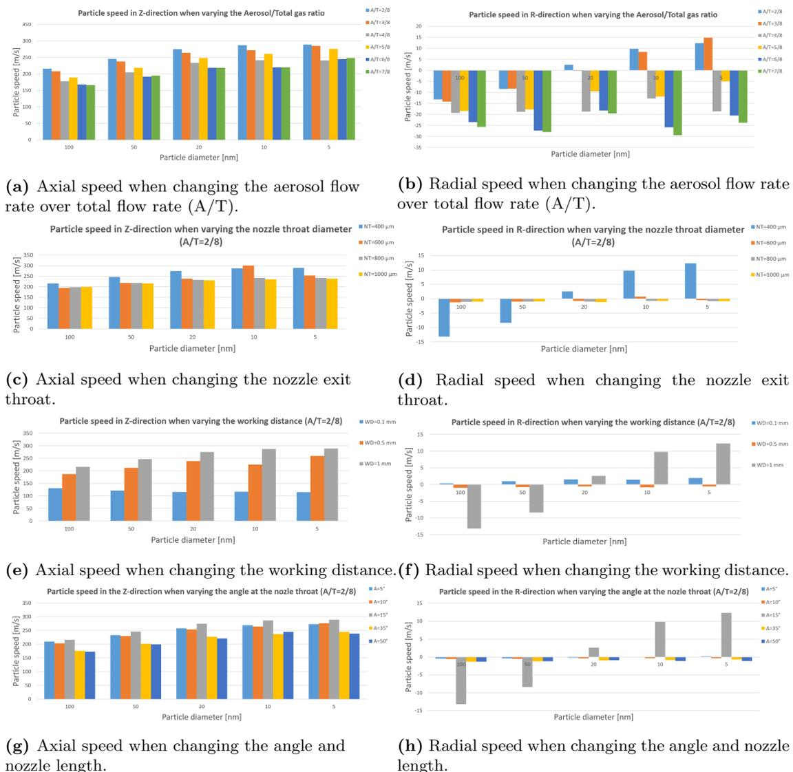
**Figure 4.4:** The particle axial (Z) and radial (R) speeds of different particle sizes when changing different parameters of a converging sheath gas nozzle. These are the maximum speeds measured at the centerline and exit of the nozzles. The values are interpolated.
