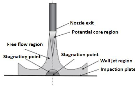
**Figure 2.2:** Schematic representation of the important components after a nozzle exit. [53]
