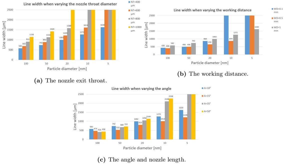
**Figure 4.3:** The line width of different particle sizes when changing different parameters of a converging nozzle. Values above 2500 microns indicate that (most of) the particles did not deposit.
