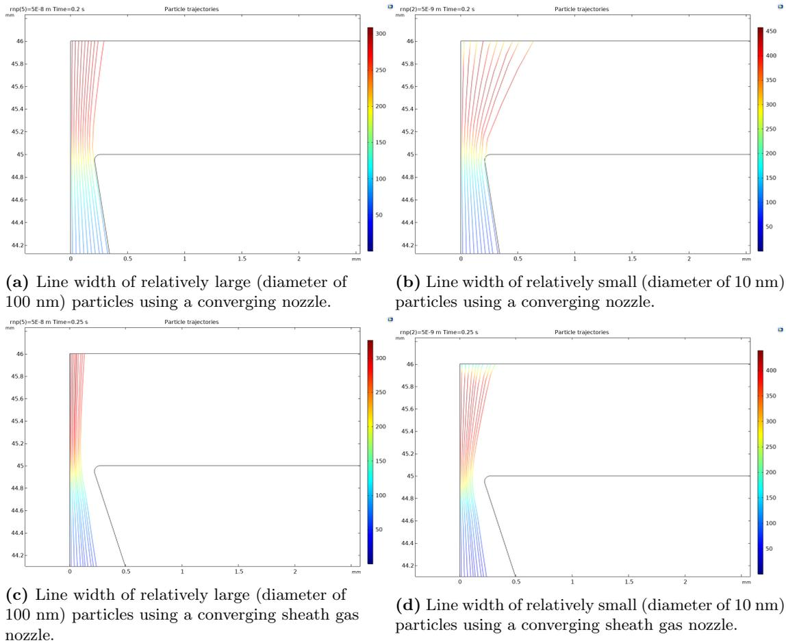
**Figure 3.15:** Typical line widths of relatively large and small particles.
