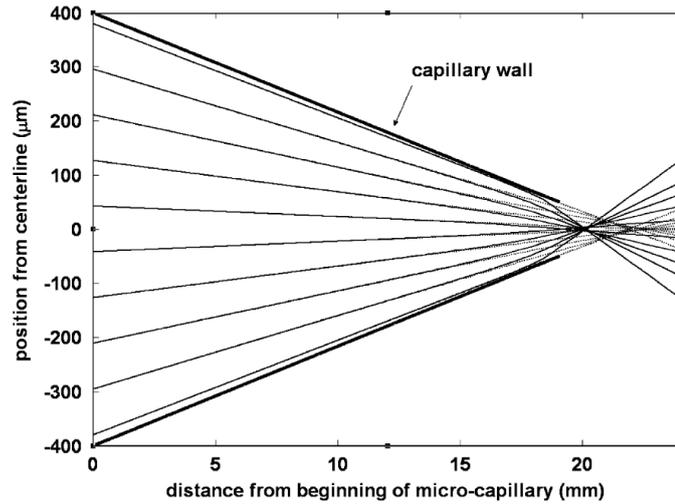
**Figure 2.14:** The trajectories of particles when starting at different positions. This is done with considering the Saffman force (solid lines) and without this force (dashed lines). [64]
