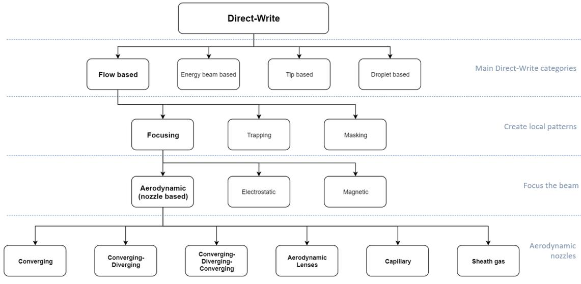
**Figure 1.1:** A compact summary chart of the direct write field, where the bold terms indicate the focus of this research.
