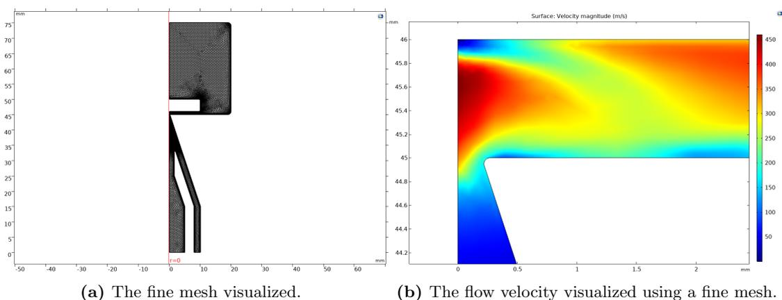
**Figure 3.8:** A fine mesh used to model the flow velocity of a converging sheath gas nozzle in COMSOL.
