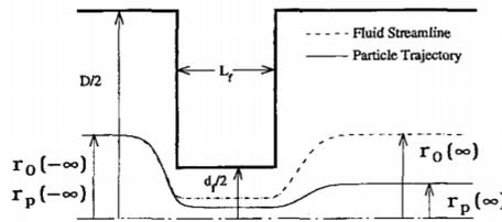
**Figure 2.1:** The contraction factor of a particle stream showed by using as an example an aerodynamic lens. [43]
