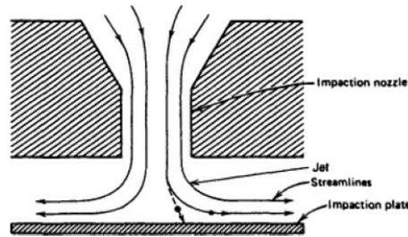
**Figure 2.4:** Streamlines are bended because the flow is deflected after the exit of the nozzle. [56]
