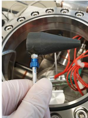
**Figure 5.10:** First connected converging sheath gas nozzle to the sheath gas pipe.
