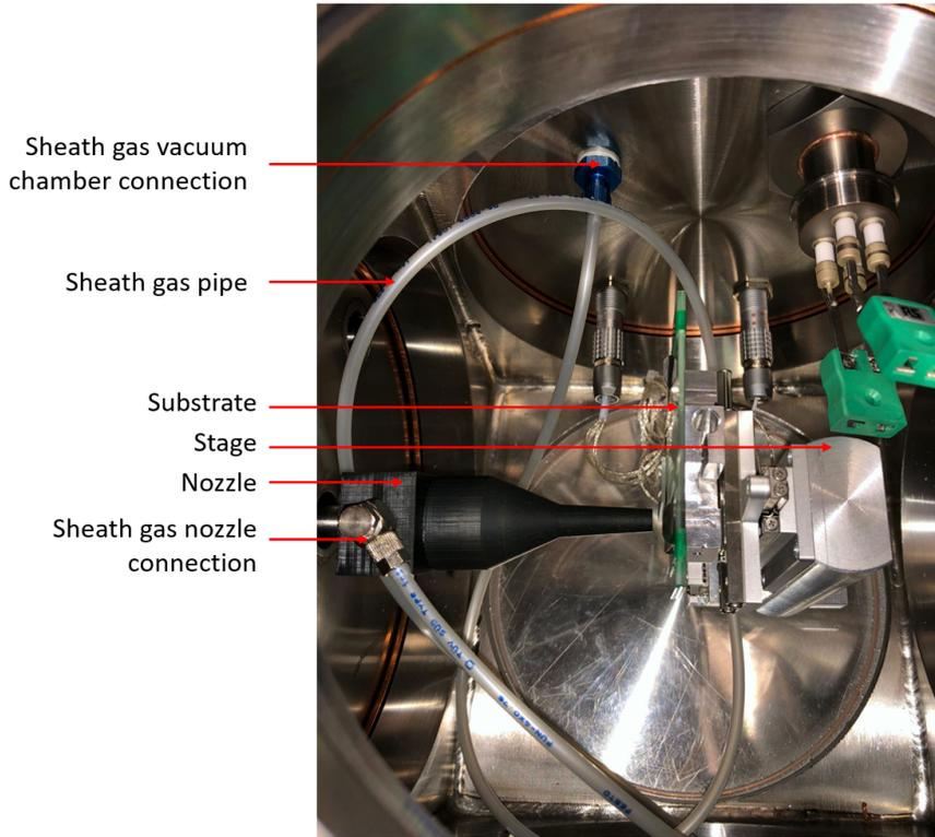
**Figure 5.8:** Converging sheath gas nozzle connected and installed in the vacuum chamber.
