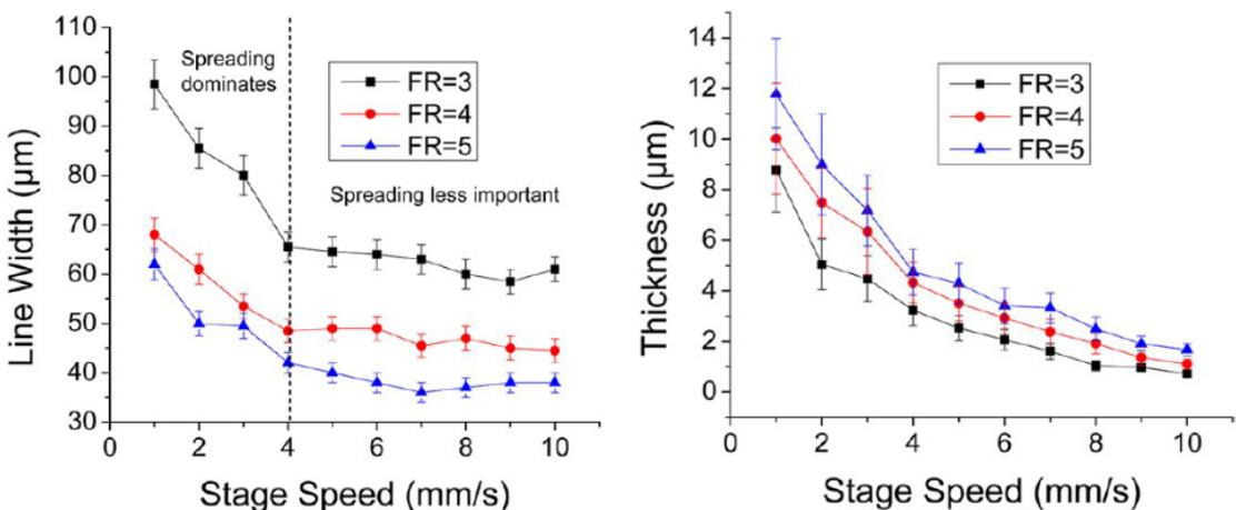
(a) Stage speed versus the line width while also considering the focusing ratio.
