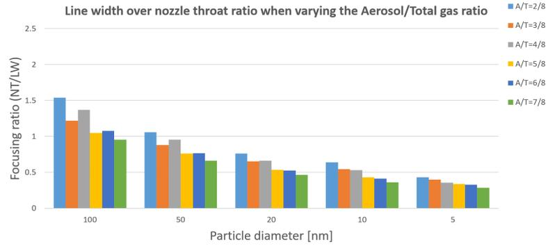
**Figure 4.7:** The focusing ratios (nozzle exit throat/line width) of different particle sizes when changing the aerosol flow rate to total flow rate ratio of a converging sheath gas nozzle.
