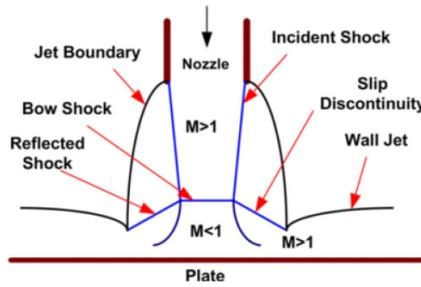
**Figure 2.3:** Schematic representation of the important components after a nozzle exit. [55]
