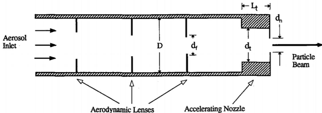
**Figure 2.9:** A schematic representation of an aerodynamic lenses apparatus. [43]
