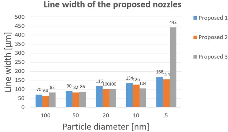
**Figure 5.5:** The line width of different particle sizes of the proposed nozzles.
