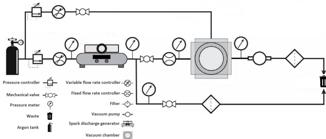
**Figure 5.7:** Schematic representation of the SAM setup with the connected sheath gas line.
