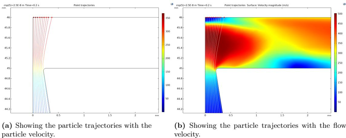
**Figure 3.11:** The particle trajectories using a converging nozzle shown in two ways. These particles have a diameter of 50 nm.
