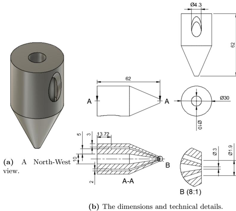
**Figure 5.9:** The first CAD model of the Converging sheath gas nozzle.
