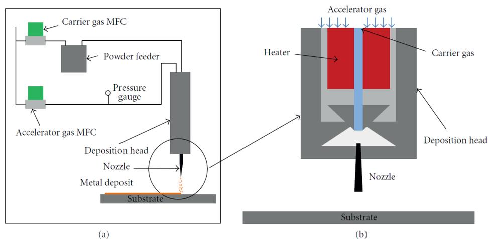
**Figure 1.2:** The Microcold spray system is shown in (a), where the deposition head of this Microcold spray is shown in (b). This schematic overview is for solid aerosols and was made by Bhattacharya et al. [20]
