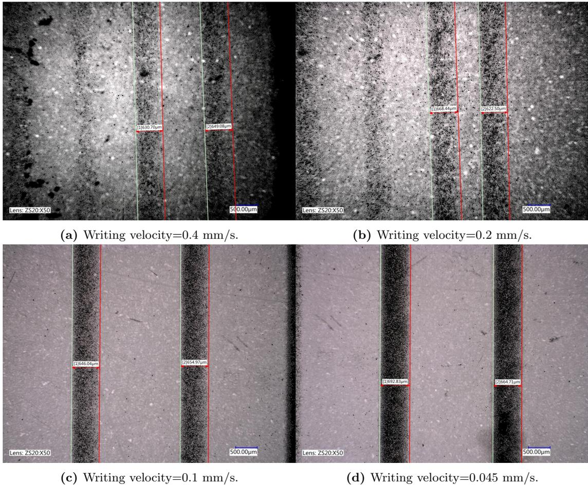
**Figure 5.16:** Digital microscope imaging showing the printed lines with different writing speeds, using a converging nozzle. The line widths shown have an error margin of  $\pm 25$  microns.
