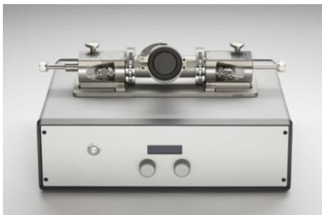
**Figure 1.4:** A spark discharge generator that is also used at the Precision and Microsystems Engineering department in Delfts University of Technology. [24]
