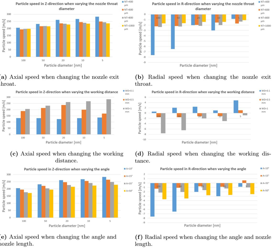
**Figure 4.1:** The particle axial (Z) and radial (R) speeds of different particle sizes when changing different parameters of a converging nozzle. These are the maximum speeds measured at the centerline and exit of the nozzles. The values are interpolated.
