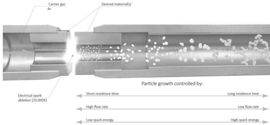
**Figure 1.5:** Generation of (nano)particles using the spark discharge generator used in the setup at the Precision and Microsystems Engineering department in Delfts University of Technology. [24]
