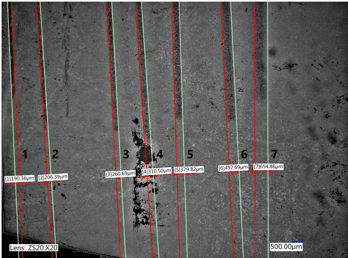
(a) Digital microscope imaging: 1)  $A/T=1/10$ , 2)  $A/T=1/8$ , 3)  $A/T=2/8$ , 4)  $A/T=3/8$ , 5)  $A/T=4/8$ , 6)  $A/T=5/6$  and 7)  $A/T=6/8$ . The line widths shown have an error margin of  $\pm 25$  microns.
