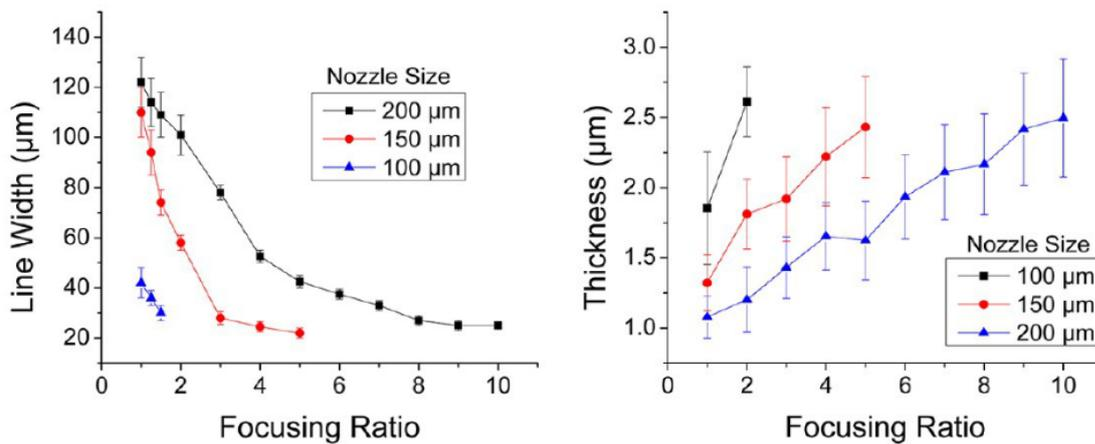
(a) Focusing ratio versus the line width while considering the nozzle size.
