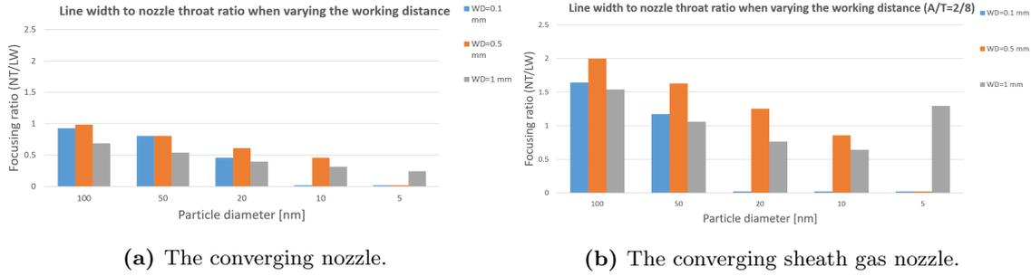
**Figure 4.9:** The focusing ratios (nozzle exit throat/line width) of different particle sizes when changing the working distance of a converging and converging sheath gas nozzle.
