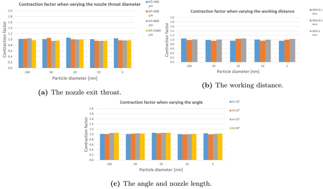
**Figure 4.2:** The contraction factor of different particle sizes when changing different parameters of a converging nozzle.
