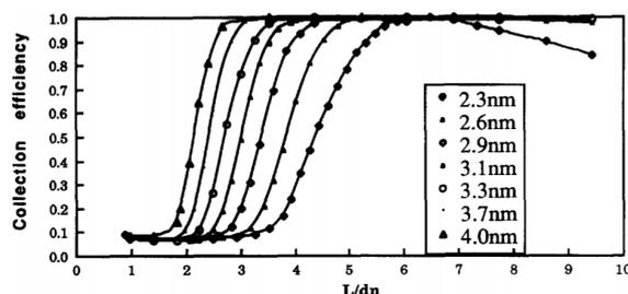
**Figure 2.6:** The collection efficiency  $\eta$  versus the nozzle-to-plate distance divided by the particle diameter  $\frac{L}{d_n}$ . [57]
