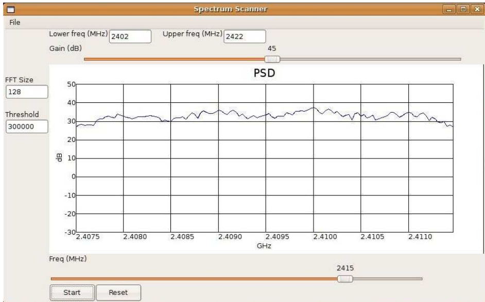
Figure 2.11: Graphical User Interface of the spectrum scanner of the AAF platform.
