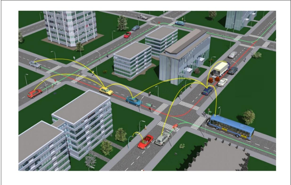
**Figure 1-1: Vehicle - Vehicle Communication Systems [1]**
