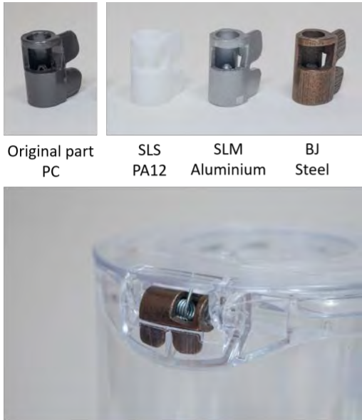
Figure 4. The spring clip printed in various materials. Limiting criteria that apply are marked with red X'es.
