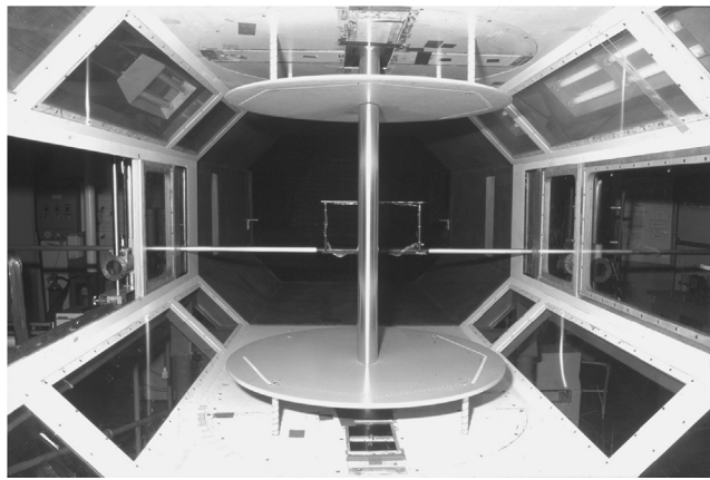
FIGURE 4.13 A test setup using a balance system. Tables are used to avoid interference between boundary layers of the tunnel walls and the model.
