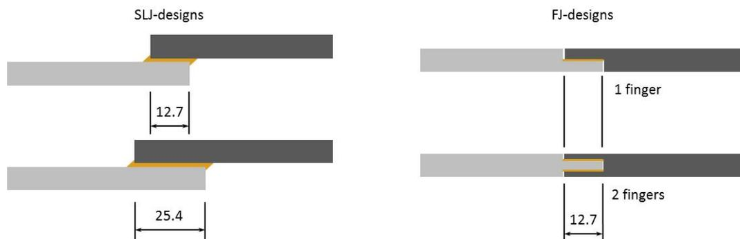
**Figure 1:** SLJ-designs and. FJ-designs tested.
