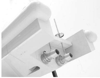
Figure 4.22: View of the waterjets arrangement of the NH-1816 model.
