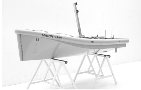
Figure 4.9: Picture of the SAR NH-1816 craft model at MARIN facilities.
