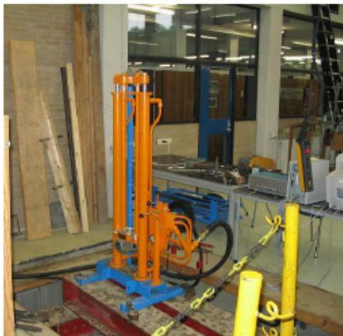
Figure 3.26: The constant loading rate apparatus
