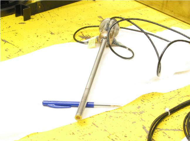
Figure 5.6: The model pile
