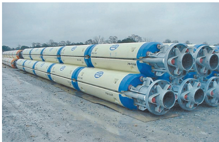
Figure 2-5 Offshore drilling riser with buoyancy modules.
