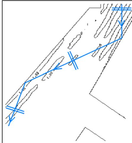
Reflection will be an important aspect to take into account when reviewing the wave conditions at the entrance. There is considerable variation in isolines, which indicates standing waves across the container port entrance. At locations close to the breakwaters, wave heights higher than the incident wave heights occur due to (almost complete) reflection. The direction of the (reflected) wave propagation in-port is clearly visible in the simulation runs.
