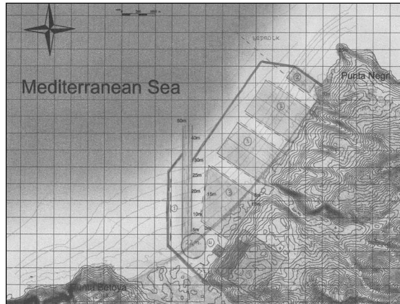
In the alternative above, to avoid towing of the liquid bulk vessels over a large distance, the liquid bulk berths are located close to the entrance, as advised in 4.3.2. However, they are now not upwind of other terminal activities anymore, and not in a secluded basin. Besides this, the tank farm (which should be located near) lies close to the fault zone around Punta Betoia which is considered less safe.
