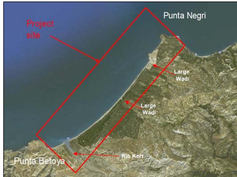
Although no exact hard boundaries for the project site (inland as well as seawards) have been specified (only the indication above), they are mainly determined by practical limits: the terrain has a rather steep slope which makes construction of the terminals and breakwaters very expensive when situated far from the coastline. This will be clarified at the end of this paragraph. First of all, the main features of the project location are described below.
