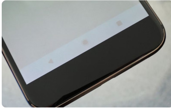
Figure 4.2: Example of OLED burn-in [32]
