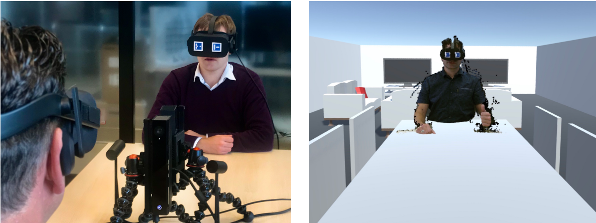
Figure 1.2: Test setup of the TogetherVR platform introduced by Dijkstra-Soudarissanane et al. [12]. In this case, two HMD-wearing subjects are captured with RGB-D sensors (left). In turn, the subjects are placed in a shared virtual environment (right). For testing purposes, the two subjects are located in the same physical space.
