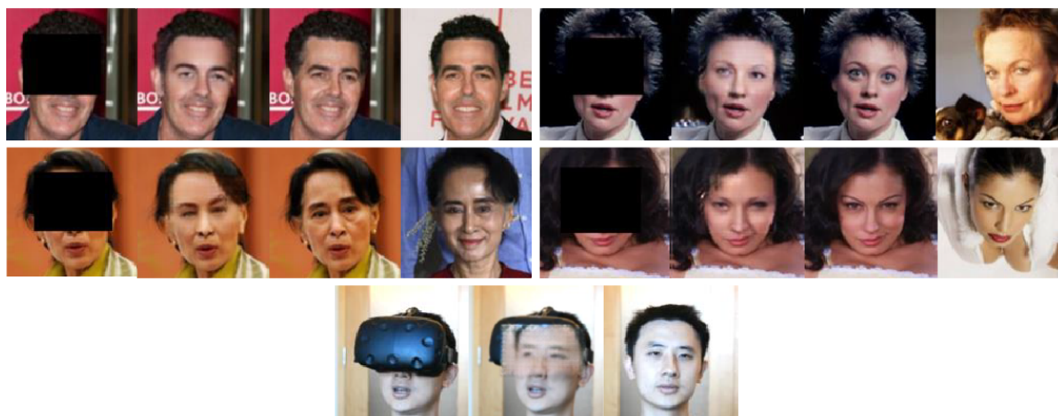
Figure 2.3: Results of RGB image inpainting method for HMD removal by Zhao et al. [36]. The top two rows contain results based on the MS-Celeb-1M [54] dataset, whereas the bottom row contains an inpainting result of real-world footage. For each result set, from left to right: input, inpainted result, ground truth, reference. The input or ground truth of the bottom result is not provided, but can be identified based on the inpainted result.
