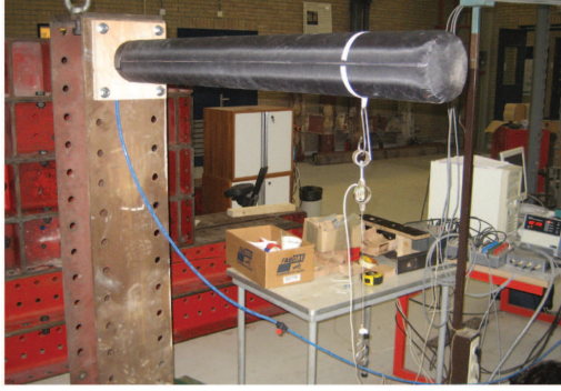
(a) Set-up to measure the inflatable beam stiffness properties.
