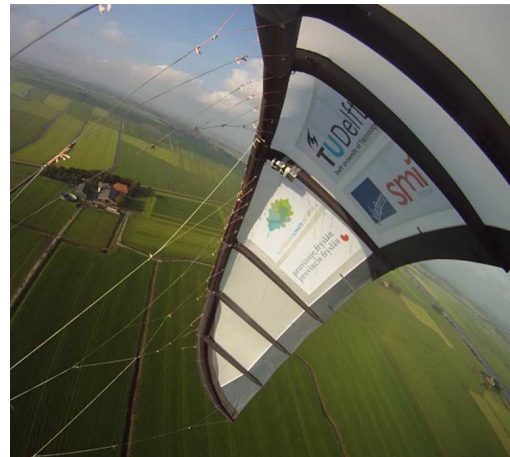
Figure 2-11: Bridle system of the Mutiny kite.
