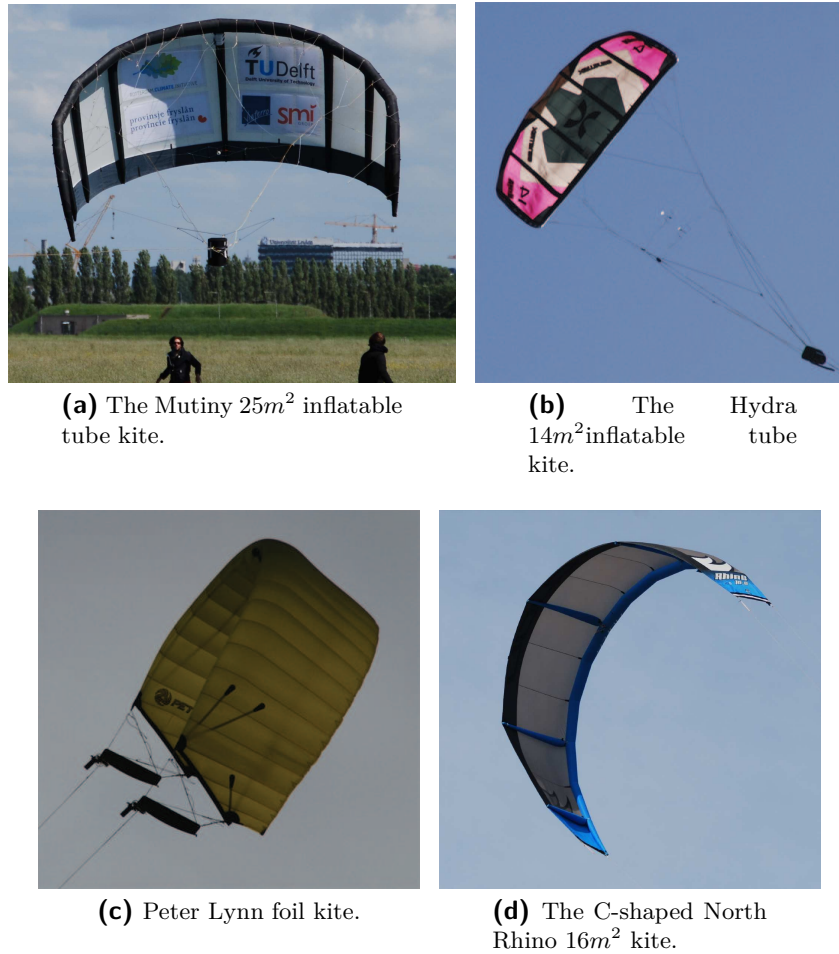
Figure 2-7: Different kite types.
