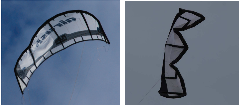
Figure 5-6: Buckling of a kite under high loading.
