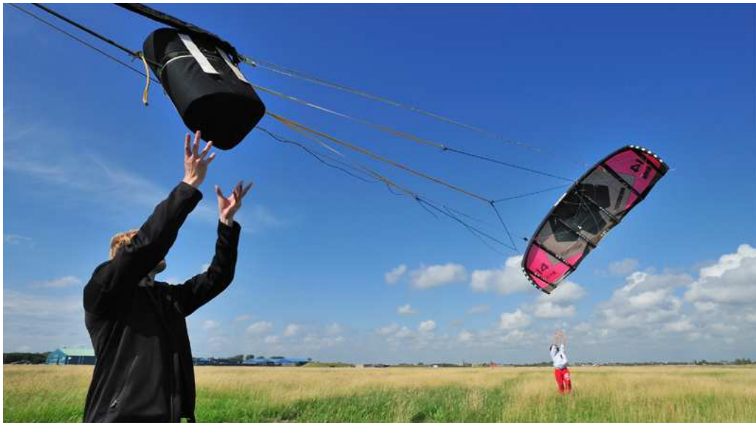
Figure 1-2: The kite power concept from the Delft University of Technology. Photo by Max Dereta.
