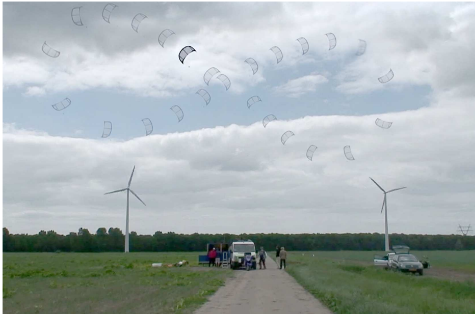
Figure 2-4: Figure eight manoeuvre during a cross wind flight.
