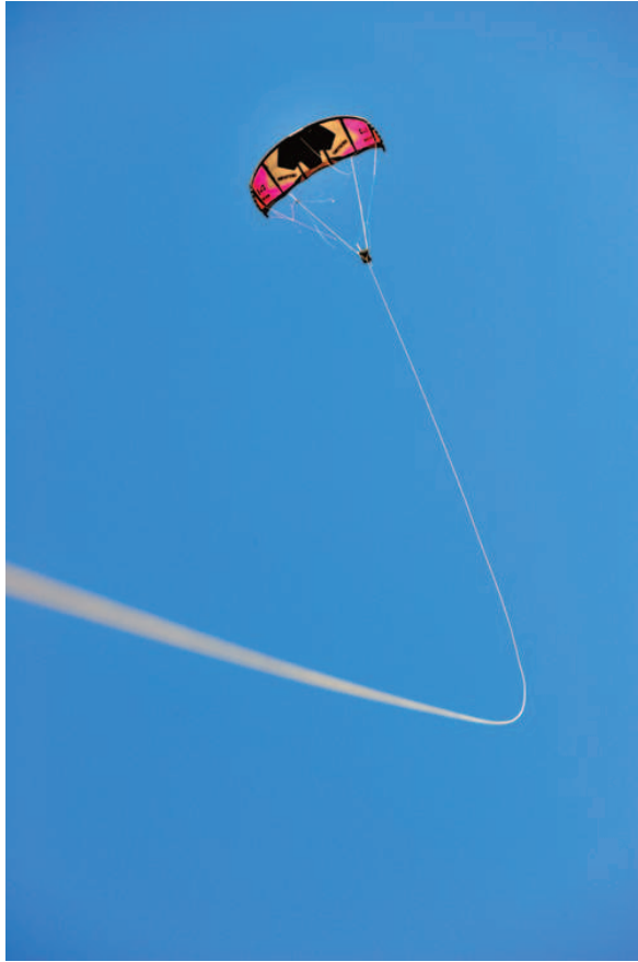
Figure 2-13: Extreme sag of the tether (photo by Max Dereta).
