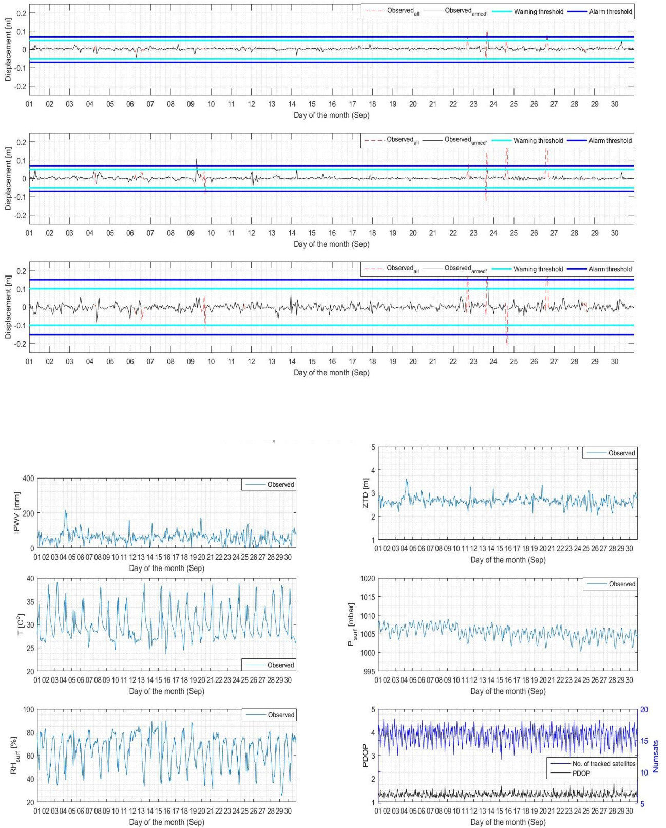
Figure A.6.2: Graphs visualizing the IM displacements (top), and the Tropospheric information, PDOP values and number of tracked satellites (bottom) as observed by the SLYG CORS during September 2016. For a more detailed explanation of the graphs, see 'Appendix 6 and Appendix 7 Figures explained'.
