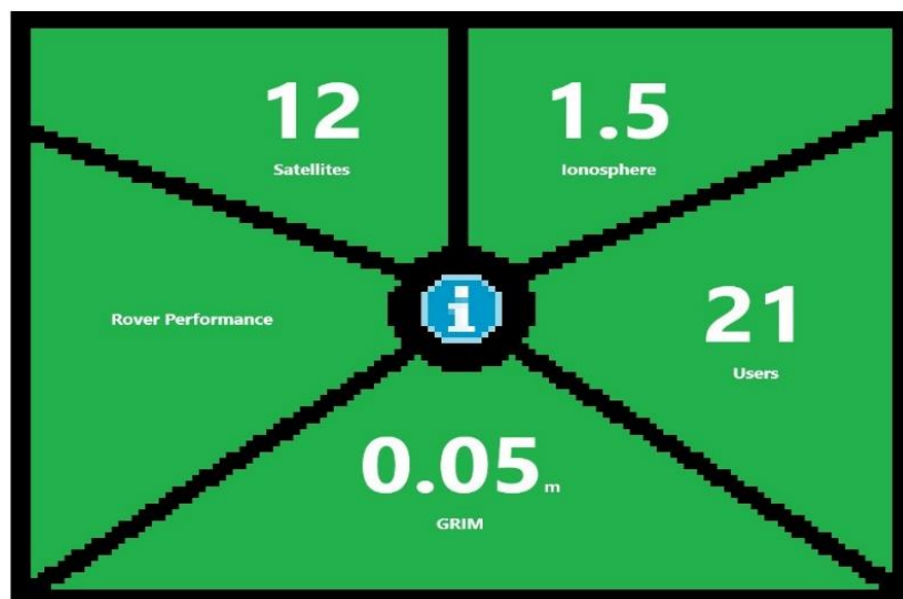
Figure 5.2: Example of what the SiReNT Dashboard could be looking like, based on the 5 parameters: the number of tracked satellites, the number of users, the GRIM (in cm), the Rover performance, and an indication of the Ionospheric delay. In the visualized situation all parameters are satisfying the set limits.
