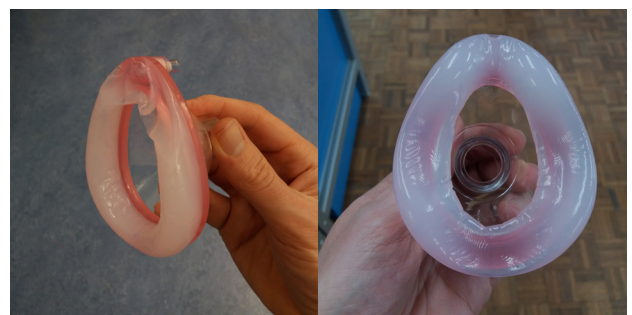
Figure 91. Filling the mask with less silicone to evaluate the surface tension.
