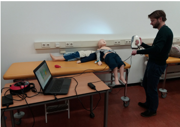
Figure 75. 3D scanning the mannequin's face with the Artec Eva.
