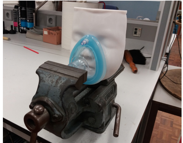
Figure 90. Silicone curing on a 3D printed face in a vice.
