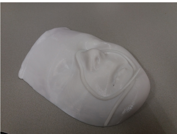
Figure 81. Test with PCL, the deformable material of the Deformable Mask.
