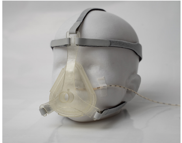
Figure 87. The Modular Mask tailored for an enriched statistical shape model of a one year old child.
