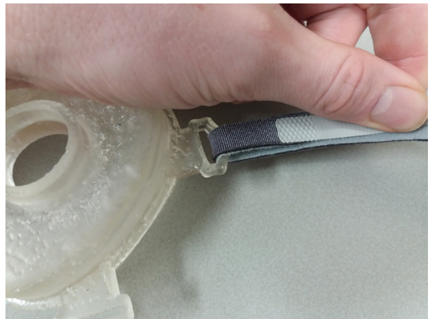
Figure 78. Flexible connection of the Flexible Mask prototype.
