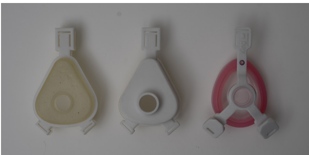
Figure 77. Removing the support material of the cushion.
