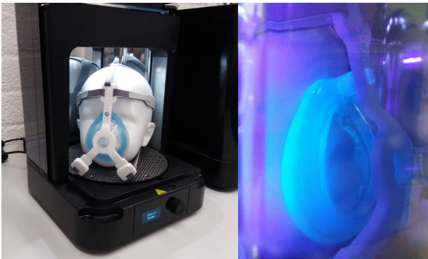
Figure 88. UV curing of Elastic Resin.
