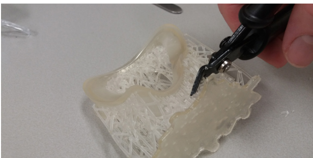
Figure 76. Removing the support material of the cushion.
