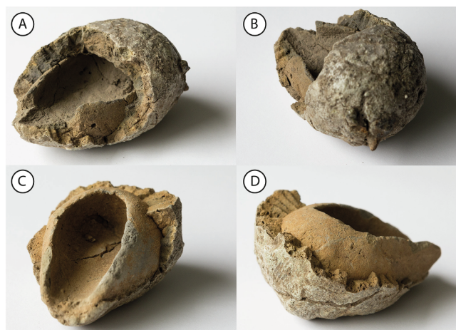
Fig. 2. Photographs of two broken crucibles (A, B #3; C, D # 13), showing the cradle inside a mantle with glassy outside. Note also the cracking pattern in the mantle.
