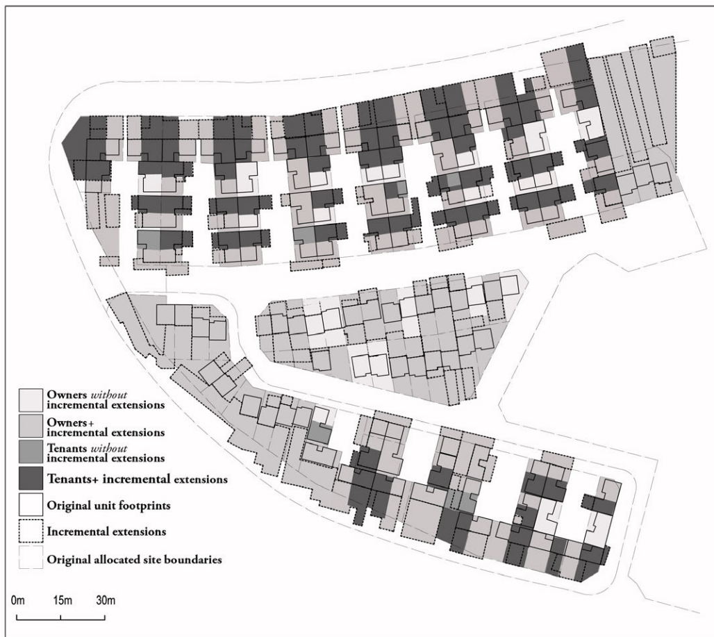
FIG. 4.3 Mapping perceived security of tenure through incremental housing extensions for Phase 1, K206
