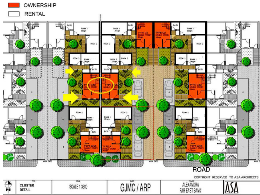
FIG. 2.16 Architectural Plans of K206 showing ownership. (Sourced from Architect Anca Szalovitz during interview (2022) and ASA Architects)
