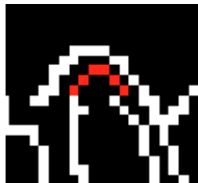
Figure 3.13: The edge is grown in the opposite direction, from left to right, between the same loose ends as in Figure 3.11b. This results in a longer connection.
