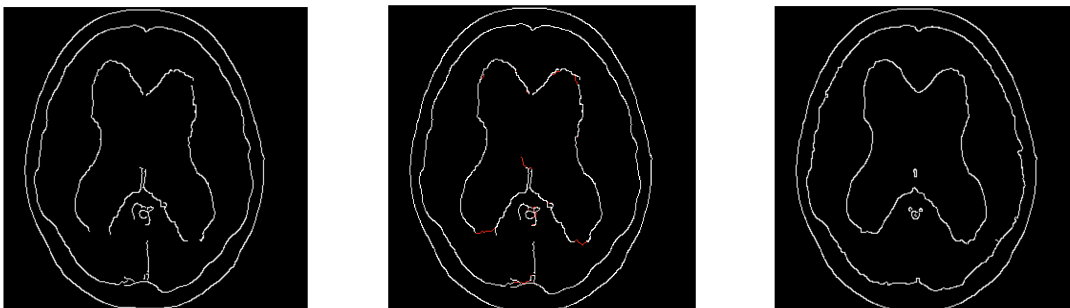
(a) Result of Canny edge detection. (b) The edges are connected. (c) Canny edge detection applied on Figure 6.1a.
