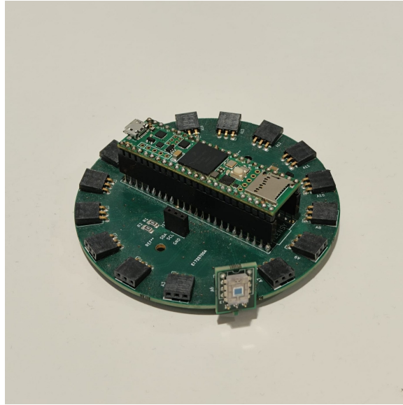
Figure 4.1: The original Teensy 4.1-based prototype board. Only one of the OPT101 photodiode boards is fitted here, though the carrier has room for sixteen.
