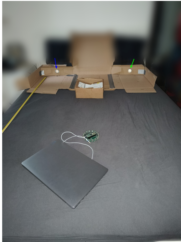
Figure 6.1: Static two-light bench setup on the original Teensy 4.1 prototype. Two lamps, marked by the blue and green arrows and modulated at 150 and 200 Hz, stand at opposite ends of the area, with the photodiode ring moved across it to map the signal. The room is otherwise dark.
