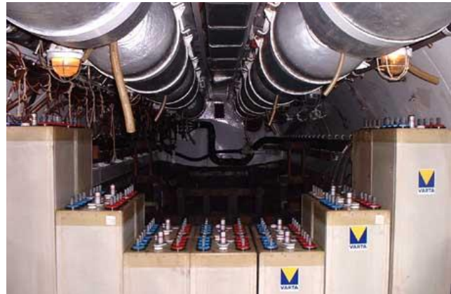
Figure 7 Multiple submarine cells forming a battery in the Tonijn [8]
