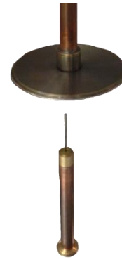
Figure 41: Final negative corona defect.
