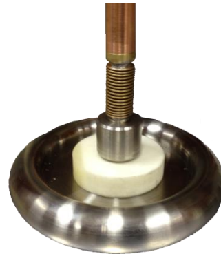
Figure 45: Final surface discharge defect.
