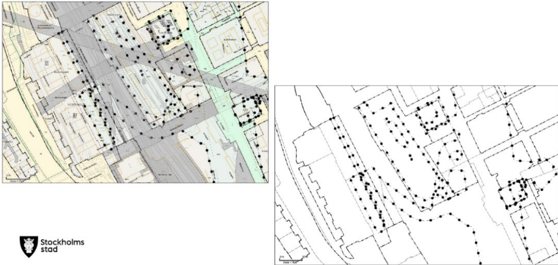
Figure 1. Selection from the cadastral index map used in the City of Stockholm. The left image includes all RRRs as well as buildings and other infrastructure, while the right image only shows real property boundaries (3D property boundaries are displayed by a filled circle on the dashed line). Adapted from Larsson, Nordqvist-Darell (2021)
