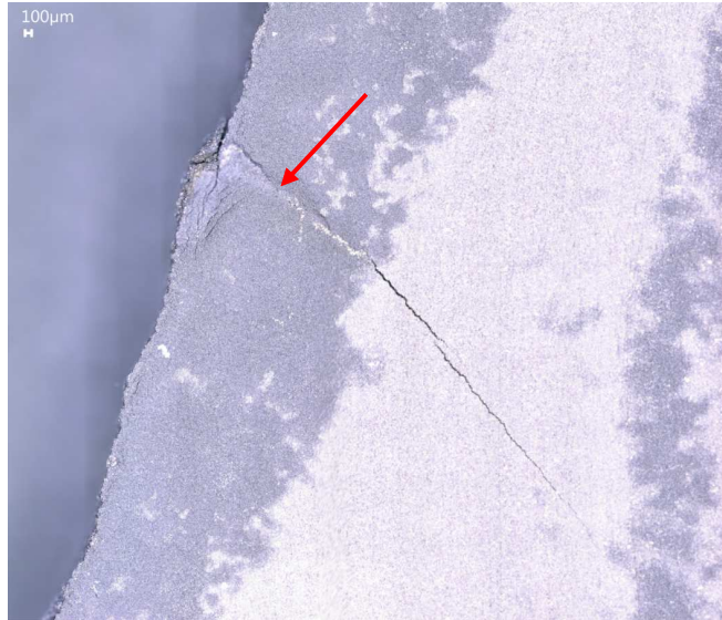
Figure 43: Optical microscopy image (Keyence) of the microcrack in \text{Ta}_2\text{AlC} wedge sample after isothermal oxidation at 600 °C for 16 hours in air, as seen from the surface (sample 150824), showing irregular oxidation.
