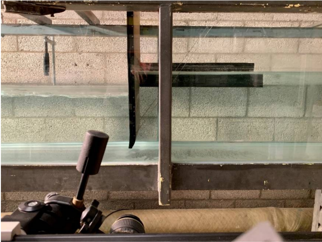
Figure 9.2: Close up photo of the underflow gate in the channel. [1]
