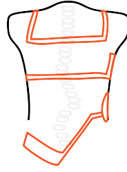
Figure 7: Schematic drawing of the TriAC brace (front view). The configuration shows the slender metal parts connecting a hip force pad with a lumbar force pad. Also a thoracic force pad is shown at the upper right side.
