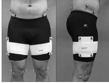
Figure 25: Marker setup used by Bruno and Jarden including four non-collinear retro-reflective markers mounted on a rigid thermoplastic plate, attached to the body using the Superwrap ™ (Fabrifoam Inc., Exton, PA, USA), reproduced from [92]
