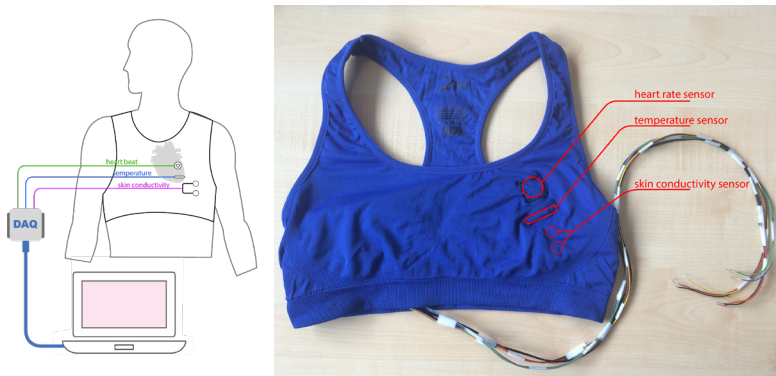
Figure 4.2. Connection of electronics (left) and placement of sensors in the garment (right). Design and photo by Xinjie Zhang.
