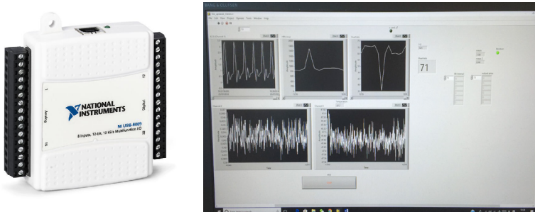
Figure 4.1. The device for data acquisition (DAQ 6009; left) and the interface of data processing software (LabVIEW; right).
