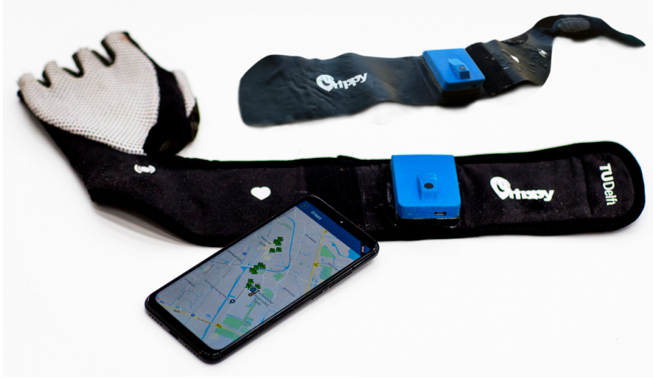
Figure 5.1. The final prototype of Grippy, which includes a glove-shaped version and a strap-shaped version connected to an app on a smartphone.
