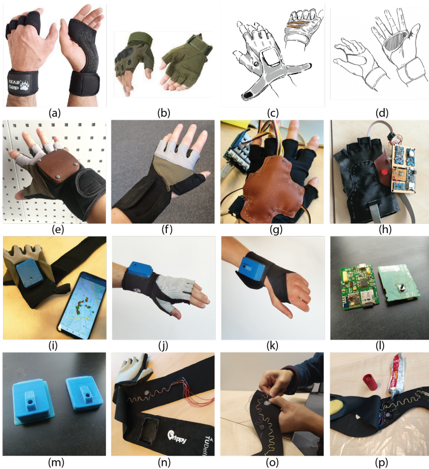
Figure 5.3. Crafting the embodiment of Grippy. The design process included inspiration sources of Grippy (a, b), conceptual sketches (c, d), Prototype 1 to Prototype 7 (e–k), printed circuit board (PCB) (l), the plastic casing to accommodate the electronic components (m), and embedding the electronics on the fabric.
