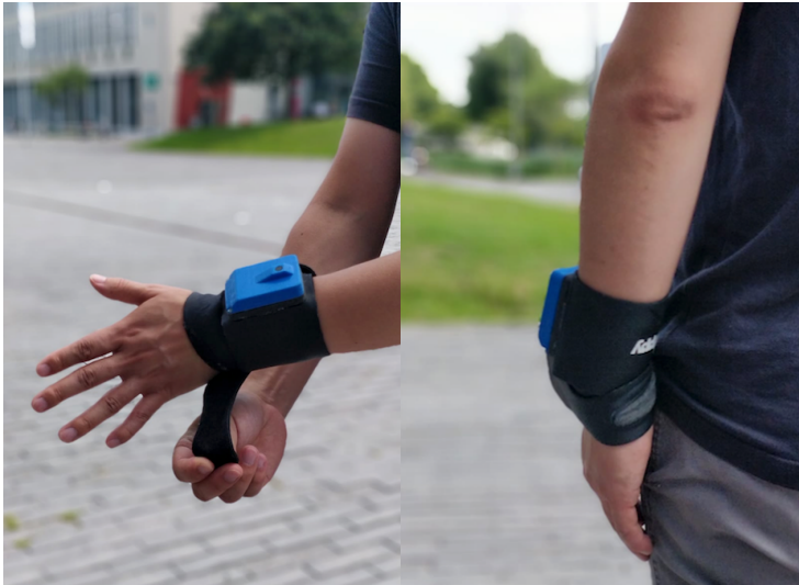
Figure 6.3. An example of how the strap-shaped version of Grippy can be worn with the haptic interface wrapped up around the wrist.
